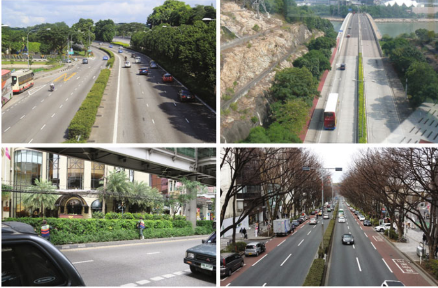
Fig. 2.6 Shrub planting in narrow planting verges in the centre divider of roads are common in cities: Singapore ( top-left ), Hong Kong ( top-right ), Bangkok ( bottom-left ), Tokyo ( bottom-right ). Apart from adding some greenness to the urban landscape, ecological functions are limited in such UGS. On the other hand, as these are often just abutting the carriageway, frequent trimming is needed, incurring high energy and carbon footprint in the process. The picture on bottom-left shows one worker trimming, and another collecting the prunings ( Photo credit P.Y. Tan )
