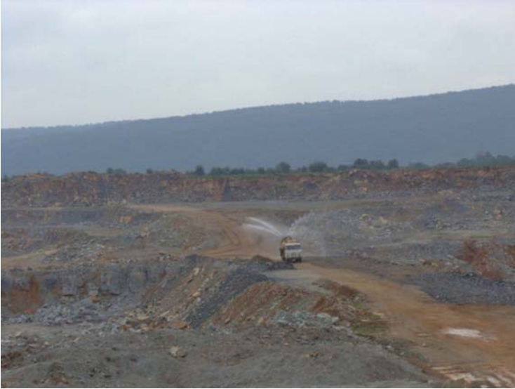
Figure 6.18 Water spraying for suppressing dust.
