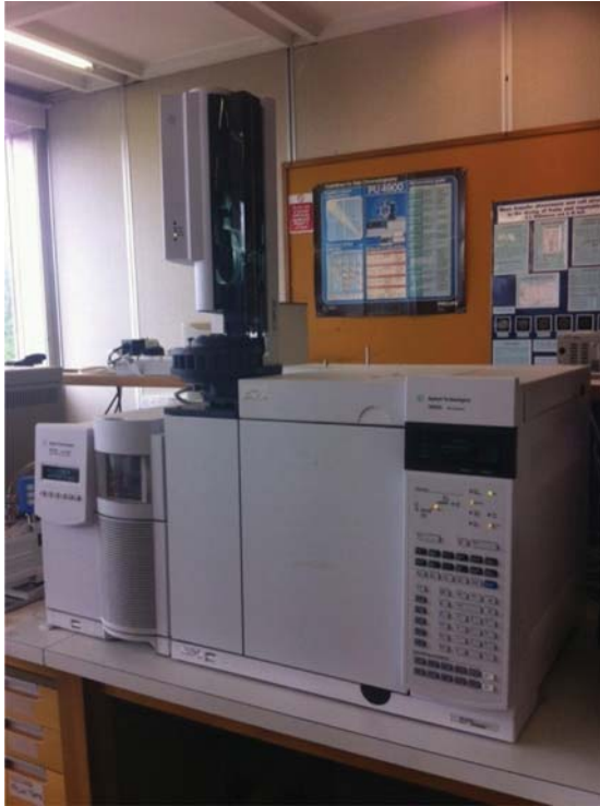
Figure 3.26 Gas chromatograph used to analyse volatile organic compounds.
