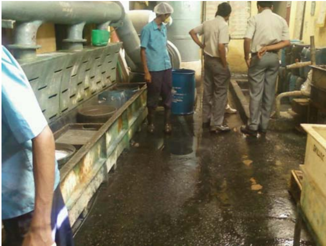
Figure 8.9 View of slippery floor.
