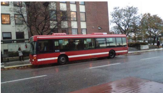
Figure 4.4 Bus fuelled by biogas generated from sewage sludge and organic solid waste in Stockholm, Sweden.
