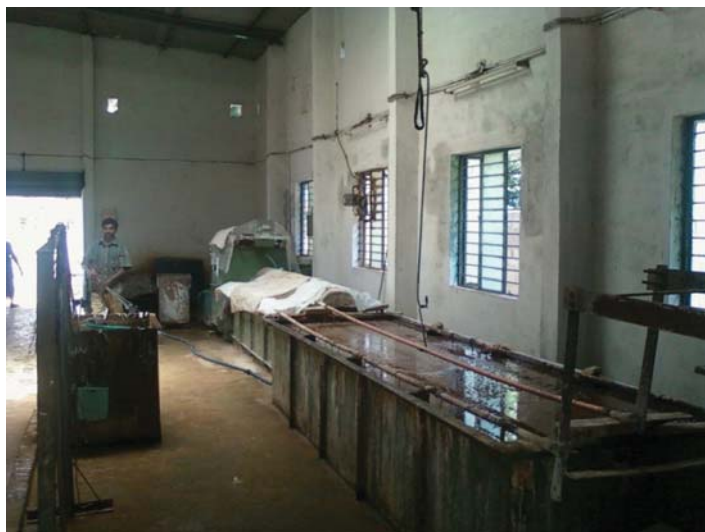
Figure 5.12 View of an electroplating unit.
