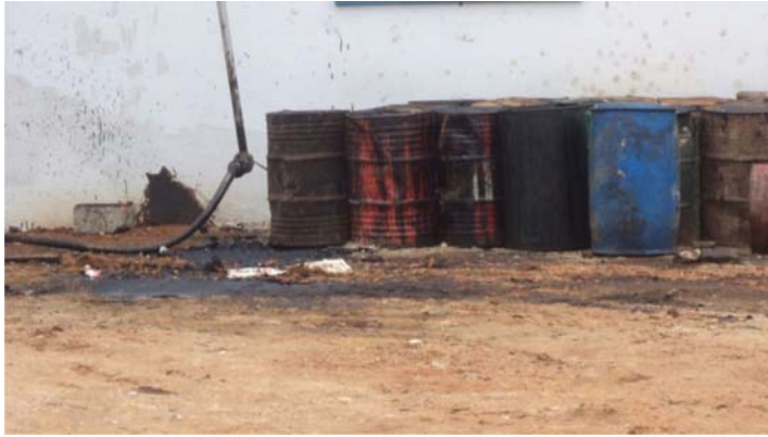
Figure 1.20 Oil spillage in a waste-oil storage yard.
