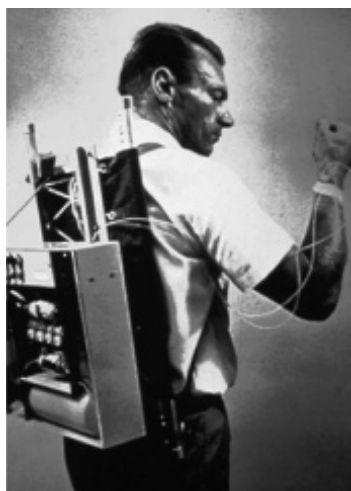
Figure 8.46 Dr. Arnold Kadish of Los Angeles, California, devised the first insulin pump in the early 1960s. Source: Medscape.
