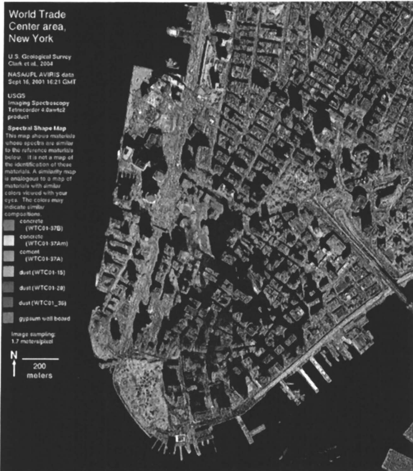
Plate 4. Map showing the WTC dust and debris plume as detected by AVIRIS indicating an asymmetry in the dust and debris distribution, with more iron bearing materials to the south by southeast. (See page 6 of color inserts.)
