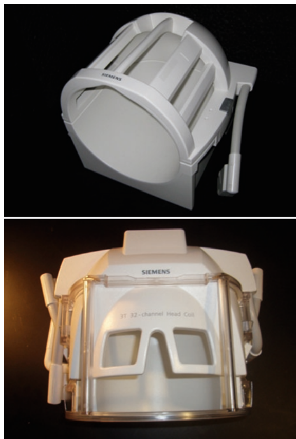
Fig. 2.21 Two examples of volume array head coils. On the top is a 12-channel unit with a 32-channel unit on the below . Preamplifiers for each channel are located at the back of the housing for improved receive signal-to-noise performance (Siemens AG Medical Solutions)
