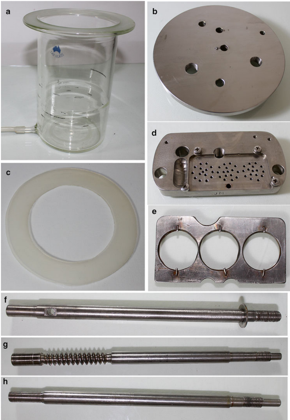
Fig. 1 Bioreactor components: (a) bioreactor vessel, (b) head plate, (c) head plate gasket, (d) base plate, (e) tissue holding plate, (f) axle support rod, (g) drive shaft, and (h) base plate control arm
