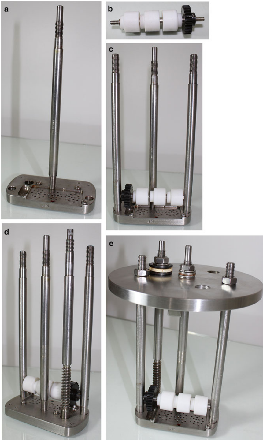
Fig. 3 Bioreactor assembly: (a) base plate control arm screwed into the middle of the base plate, (b) roller axle inserted through the three rollers with cams and worm gear, (c) roller axle mounted onto the axle support rods attached to the base plate, (d) drive shaft attached to the base plate to mesh with the worm gear, and (e) head plate fitted onto the base plate control arm, the two axle support rods, and the drive shaft using washers and screw nuts
