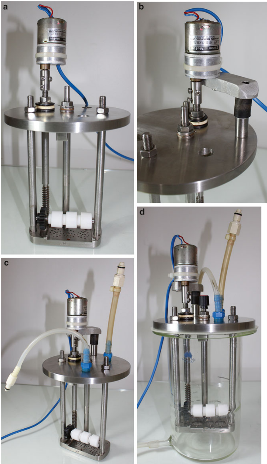
Fig. 4 Bioreactor assembly: (a) motor connected to the drive shaft using the shaft sleeve connector, (b) motor fixed to the head plate using the motor support arm, (c) silicone tubing for inlet and outlet gas streams attached to the head plate using plastic tubing adapters, and (d) marked plastic control knob attached to the top of the base plate control arm and the entire mechanical assembly inserted into the bioreactor vessel to complete the mechanobioreactor
