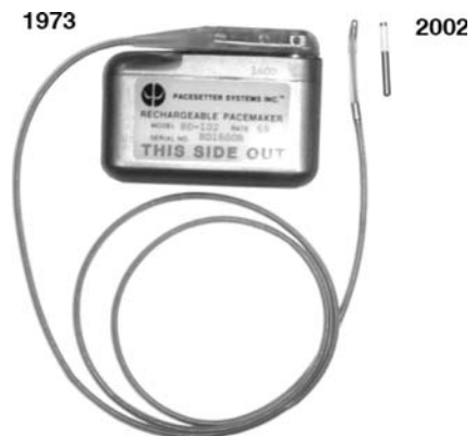
Figure 15.1 Fixed rate rechargeable cardiac pacemaker, released in 1973, next to a programmable rechargeable injectable microstimulator, released in 2002. The microstimulator can be programmed to the same stimulator parameters as the pacemaker.
