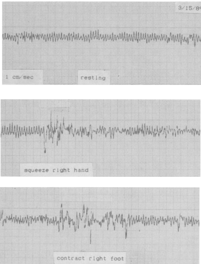
Figure 19. Microvibrations recorded from the left upper forearm using the crystal phonograph-pickup transducer mounted as shown in Figure 18.
