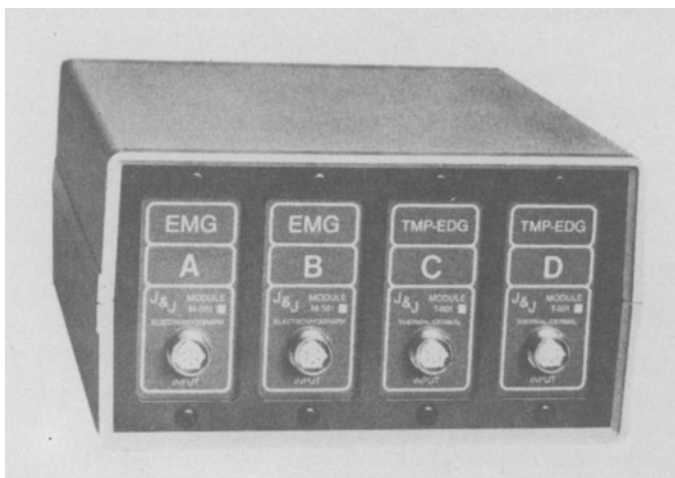
Figure 3. J & J I-330 Physiological Interface System Modality Modules.
