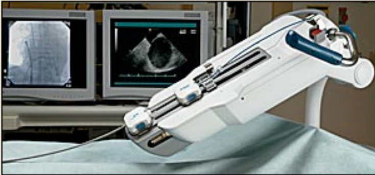
Fig. 3. Sensei robotic catheter system
