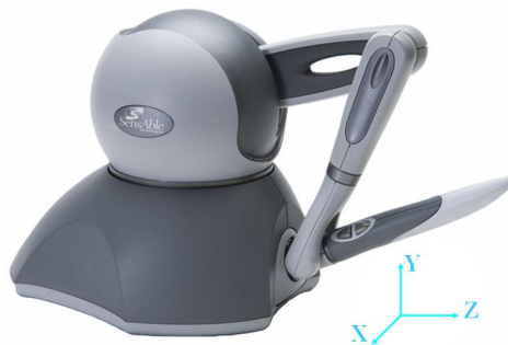
Fig. 12. Coordinate system of Phantom Omni
