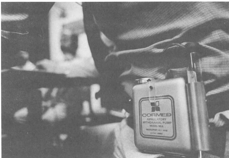
Figure 1. Cormed ambulatory withdrawal pump and blood collection tube in place on a volunteer's waist.
