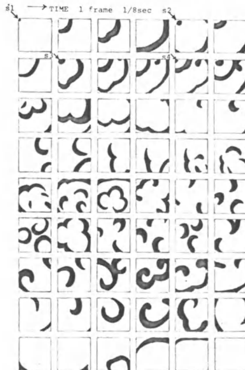
Pencil tracings at 1/8 s intervals (left to right, then down a row) from photographs of a 30 cm × 30 cm grid of 26 × 26 iron wires in nitric acid. Stimuli introduced at S 1 , S 2 , S 3 , and S 4 . Spontaneous activity persists for a while in the form of waves irregularly pivoting about moving end points. (From Nagumo et al., 1963, Figure 15, with permission.)
