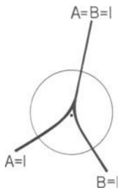
Figure 18. A locus of fixed composition, determined by at least two independent quantities, can cut a ring just once and then vanish (as A = 1 and B = 1 diverge).
