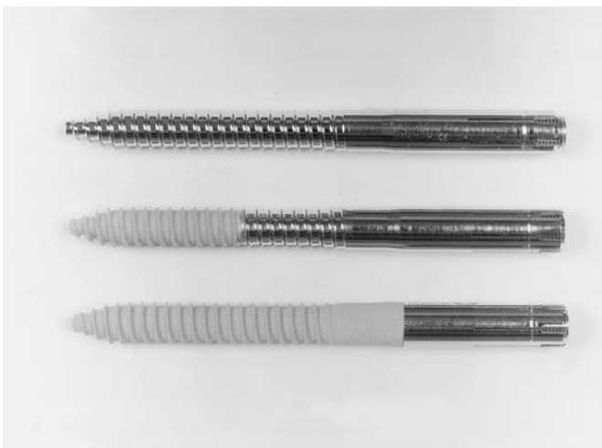
Figure 4 Stainless steel pedicle screws, 6 \times 70 mm. Uncoated (upper), partly HA coated (middle), and fully HA coated (bottom). (From Ref. 48.)
