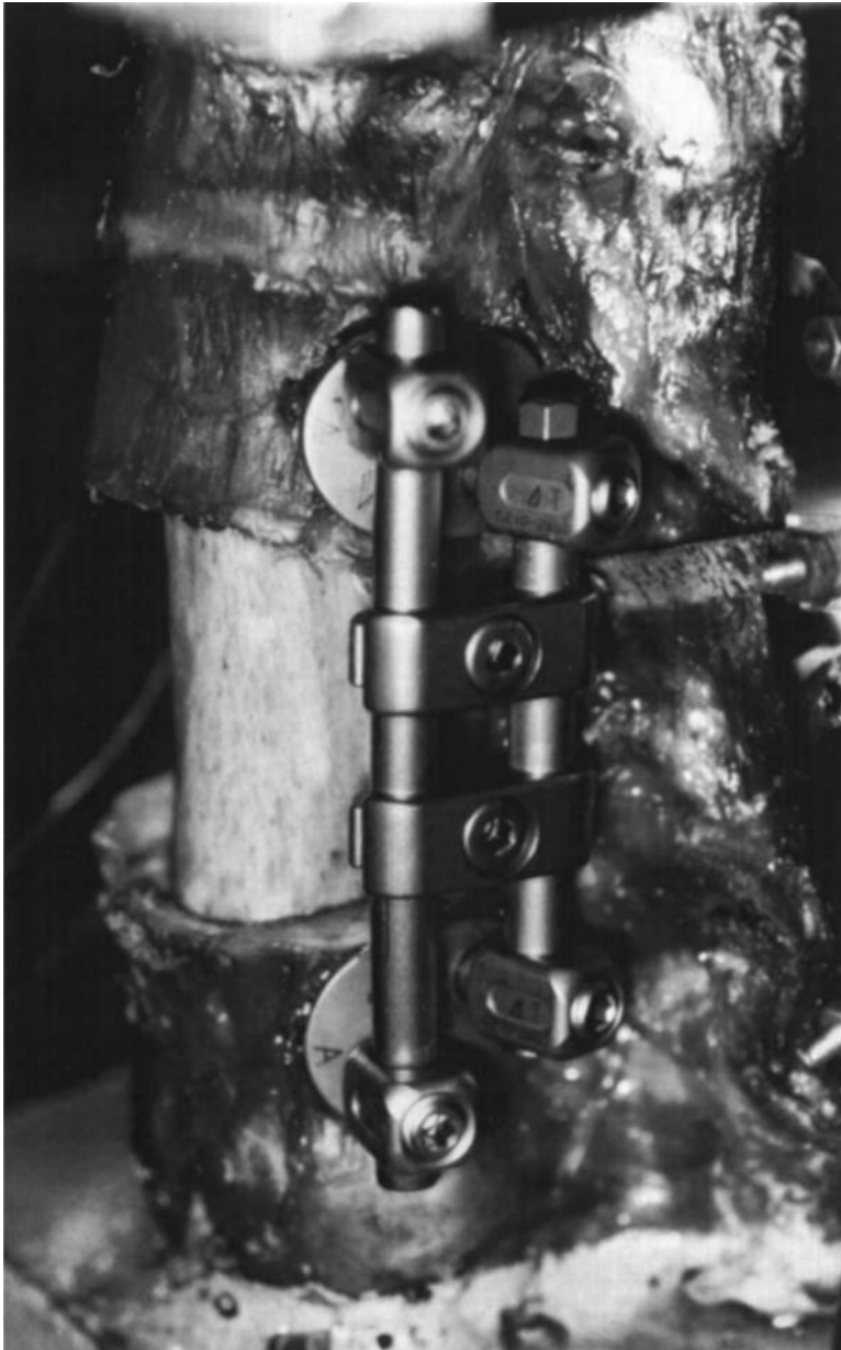
Figure 2 The SRK device applied with four bicortical screws across T12 and L2. These bone screws are constrained to the rods.
