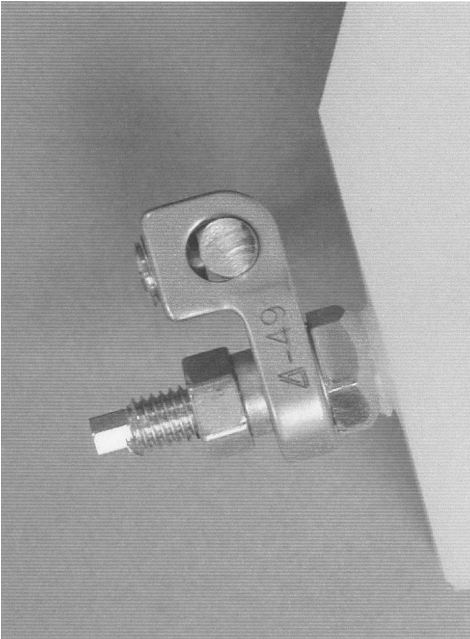
Figure 1 Custom instrumentation. A bushing machined to allow 2 mm of anterior-posterior motion along the shaft of the pedicle screw.
