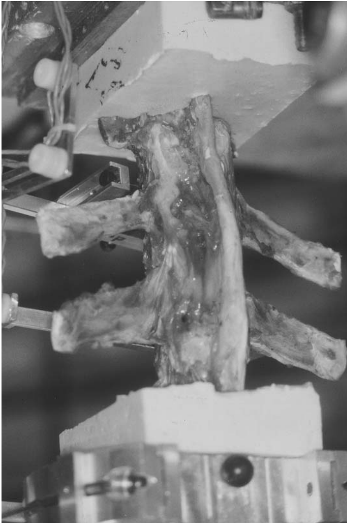
Figure 11 The spine-testing apparatus in use allowed evaluation of lumbar vertebral specimen in all six degrees of freedom (flexion and extension, lateral bending, and rotation).
