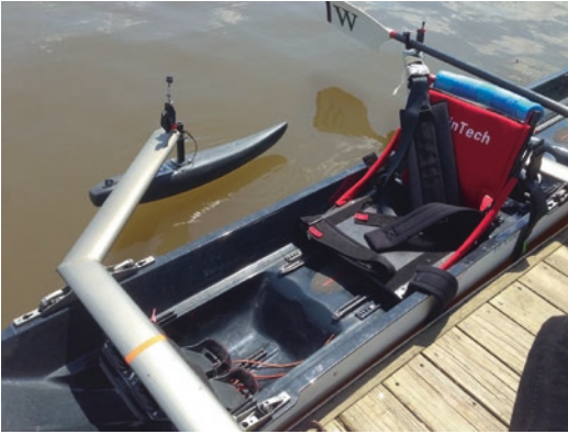
An arm/shoulder setup for a sweep rower including fixed seat and pontoon (Photo courtesy of Alan Schleier)
