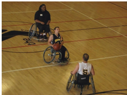
Fig. 2.3 Exemplifies the varying heights of the athlete's chairs based on position from an elevated position for the athlete in the back, left of the picture to a lower center of gravity for those athletes on the right. (Photo courtesy of Marshall Lee Tempest)
