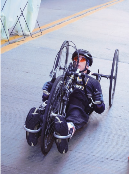
Fig. 2.13 Recumbent handcycle used for racing and exercise
