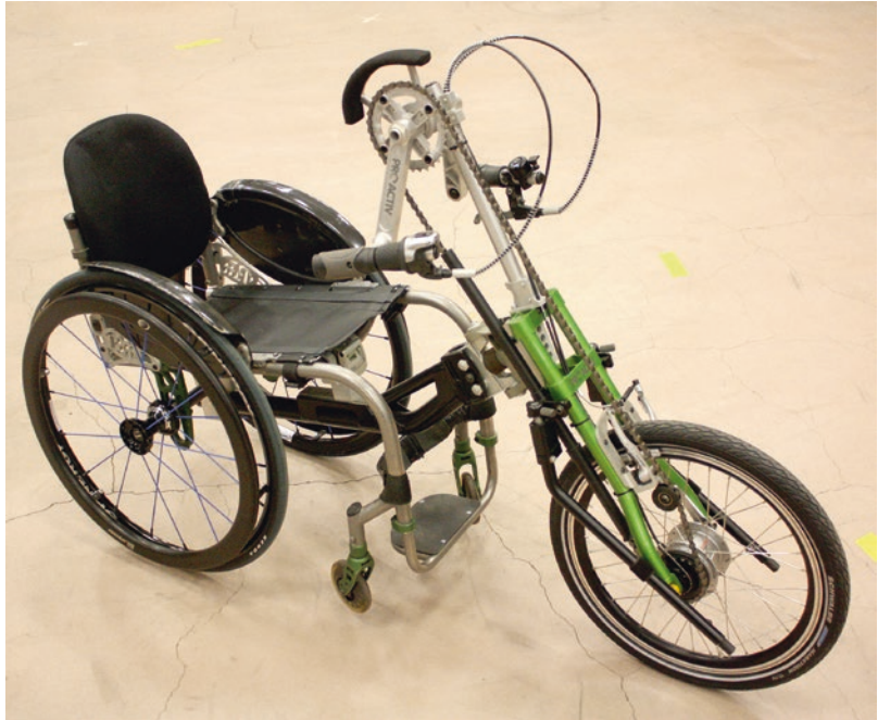
Fig. 2.12 Add-on handcycle used to convert a manual wheelchair temporarily into a handcycle for touring, shopping, and socializing
