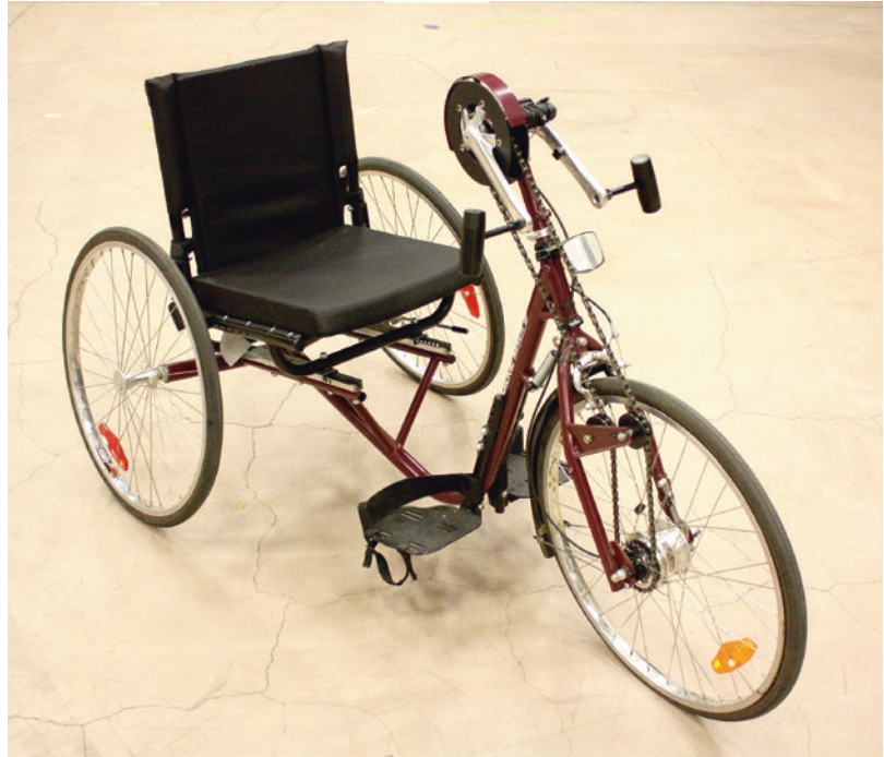
Fig. 2.11 Upright handcycle used for touring, socializing, and shopping
