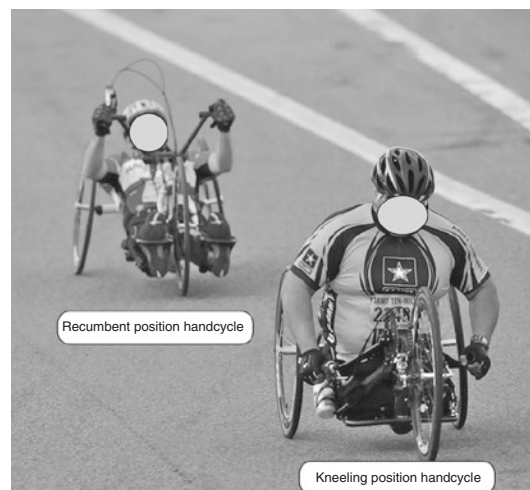
Fig. 10.1 Recumbent and kneeling position handcycles (adapted from Cooper and De Luigi, PM R 2014, S37)
