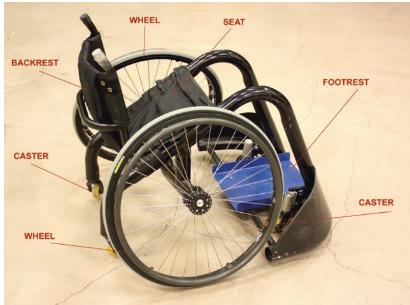
Fig. 2.1 The basic components of sports wheelchairs are the wheels, casters, footrests, backrest, and seat
