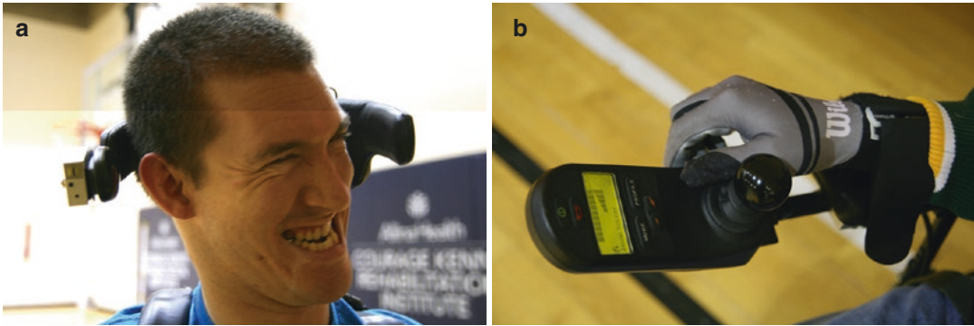
Fig. 14.6 Power wheelchair controls. Powerchairs are operated by a variety of control systems. Images a and b are two examples used by participants to play power soccer. (a) Head control: Photo credit Brionn Tonkin,
