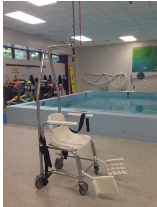
A water-friendly transfer chair with ceiling-lift suspension (Photo courtesy of Alan Schleier)
