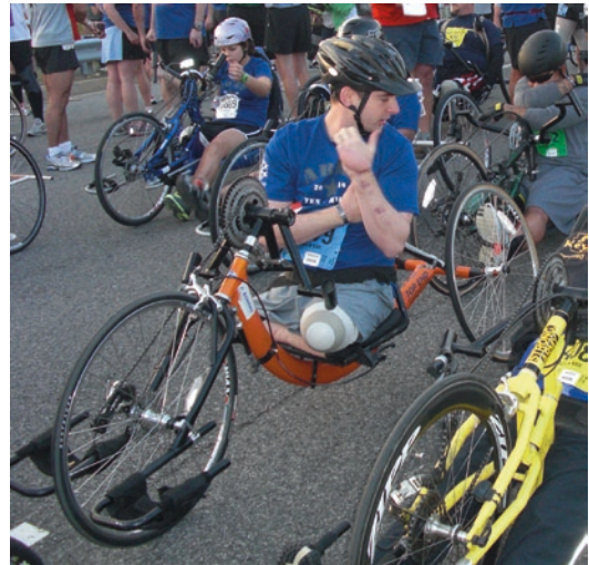
Fig. 2.14 Kneeling handcycle used for racing and exercise
