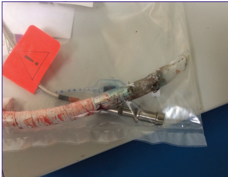
Figure 4–1. Laser Shield II endotracheal tube with cuff inflated with saline and close-up of cuff area after fire.
