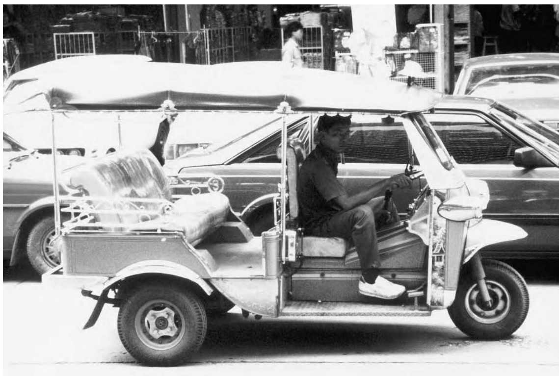
Plate 28.2 The tuk-tuk , essentially a motor scooter fitted with a rear seat and covered by a plastic-coated canopy, carries up to three passengers through the traffic chaos of Bangkok
