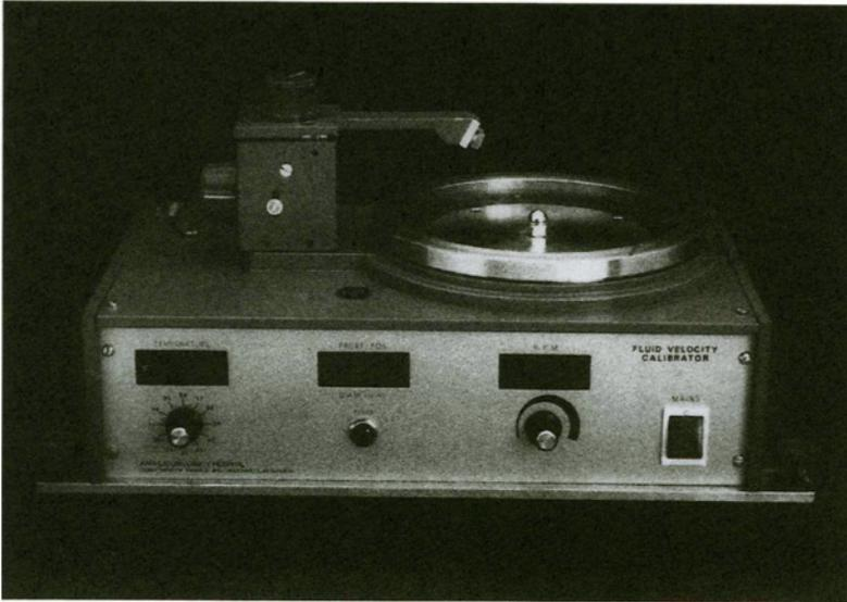
**Figure 9.** An example of a turn-table used for calibration of hot-film anemometer probes. By determining the distance from the probe tip to the center point of the turnplate and its rotational speed, it is possible to calculate the fluid velocity, applied on the hot-film.
