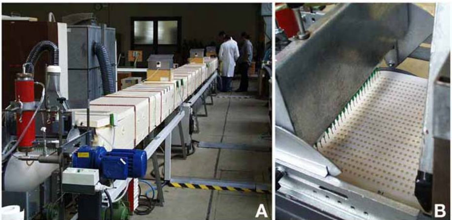
Fig. 5. Pilot-plant for continuous production of LentiKats at the Institute of Technology and Biosystems Engineering, Federal Agricultural Research Center, Braunschweig, Germany. (A) General view. (B) The multi-nozzle system puts rows of droplets onto the belt.
