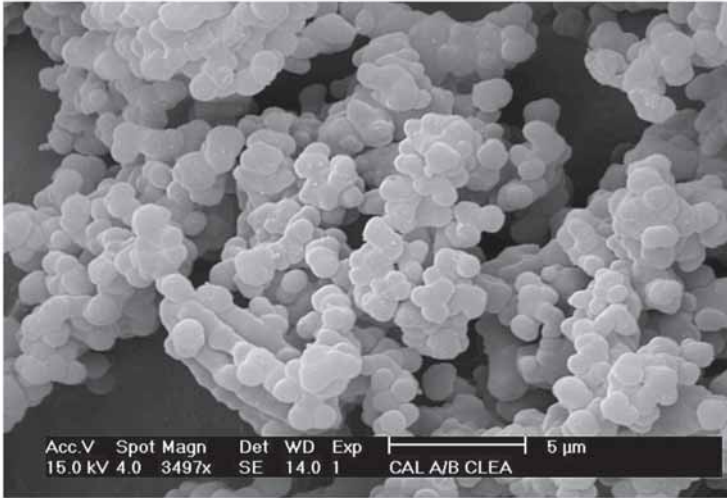
Fig. 1. C. antarctica lipase A/B CLEA. One CLEA particle can contain up to 8 million enzyme molecules (original magnification \times 3500 ).
