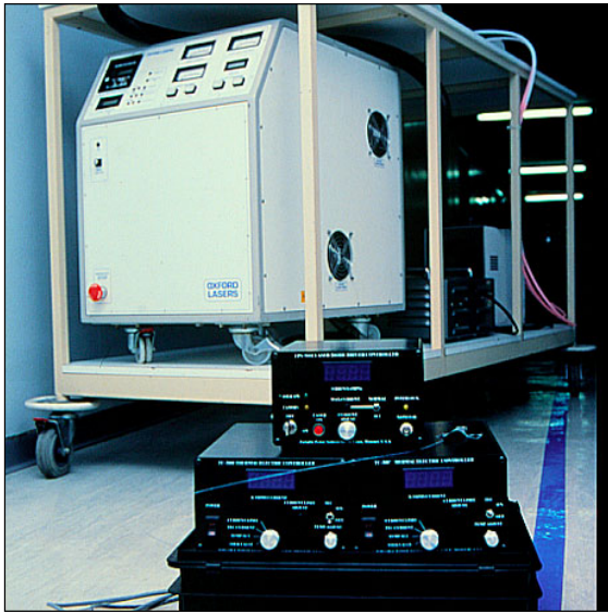
Figure 8.1 Lasers used to deliver red light at 630 nm for photodynamic therapy. Conventional large copper-vapour laser coupled to a tunable dye laser and, in foreground, prototype of new generation diode laser.
