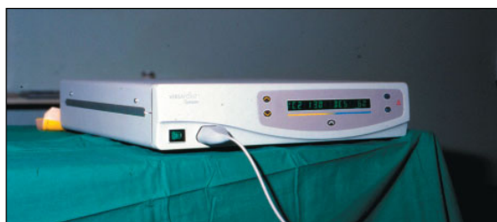
Figure 15.6 Versapoint (Ethicon, U.S.A.) 'smart' generator which automatically controls power output to the tissue impedance.
