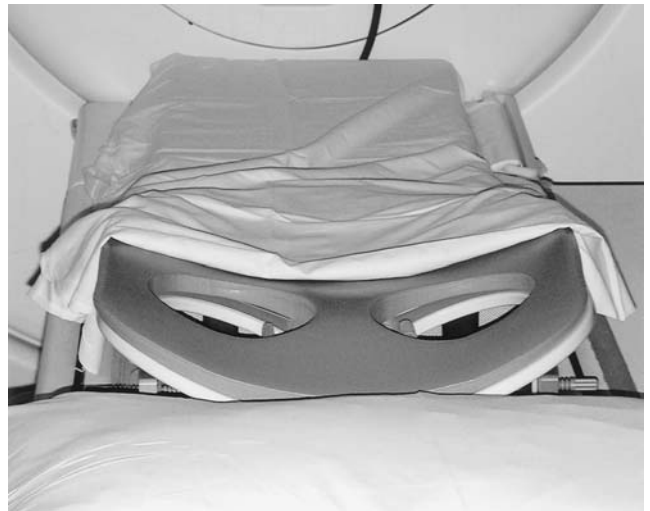
FIGURE 7.1. Bilateral breast coil (MRI Devices, Waukesha, WI) provides imaging of the entire breast, axillary tail, and excellent penetration to the chest wall. Multiple coil elements surround the breast. The coil can be used for either unilateral or bilateral imaging with high signal-to-noise ratio. Open architecture facilitates examination of very large breasts.
