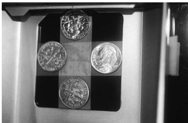
FIGURE 12.5. Collimation testing. Testing is done with four coins taped inside the compression plate biopsy opening. The edges of the coins should abut the edges of the opening on all four sides. When an image of these coins is obtained without angulation of the tube, the four coins should all be completely visualized. If not all seen completely, collimation is too tight and should be adjusted.
