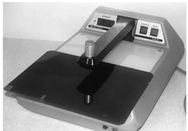
FIGURE 12.3. A densitometer is used to calculate film density in several quality control tests.
