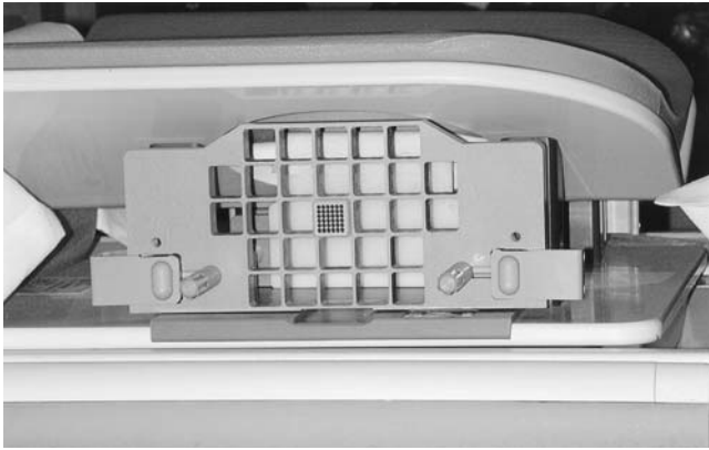
FIGURE 7.3. Compression grid plate with needle guide (Biopsy-System No. NMR NI 160; MRI Devices, Waukesha, WI).
