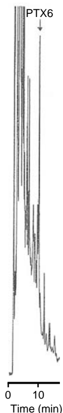
FIGURE 16.7 Fluorescence HPLC chromatogram of ADAM derivative of PTX6 in hepatopancreas of scallops. Column: Develosil ODS-5 (250 mm × 4.6 mm I.D.); Mobile phase: MeCN–H 2 O (8:2, v/v), Flow rate: 1.1 ml/min, Excitation: 364 nm, Emission: 412 nm.
