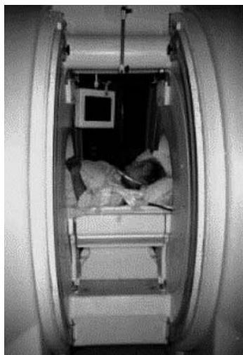
Fig. 6.1. The vertically open MRI system. The flexible radio-frequency coil is placed on the patient's shoulder when the intervention is performed. The liquid crystal display monitor inside the gap provides MR images during procedures
