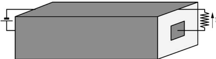
FIG. 3.1. Infinitely long coaxial cable carrying a stationary surface current.
