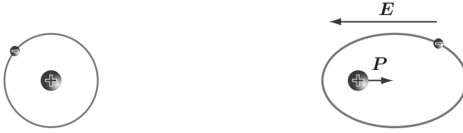
Figure 1.1: Dislocation of local charges by an exterior electric field \mathbf{E} and the polarisation field \mathbf{P} (without (left) and with (right) exterior electrical field).
