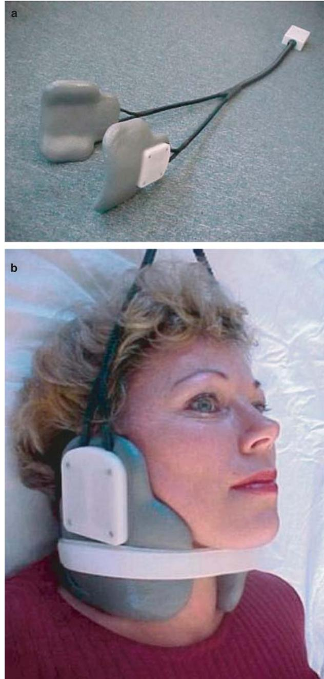
**Fig. 4.** Four-channel phased array surface coil dedicated to carotid imaging to maximise signal to noise at a  $12 \times 12$  cm field of view (Flick Engineering).
