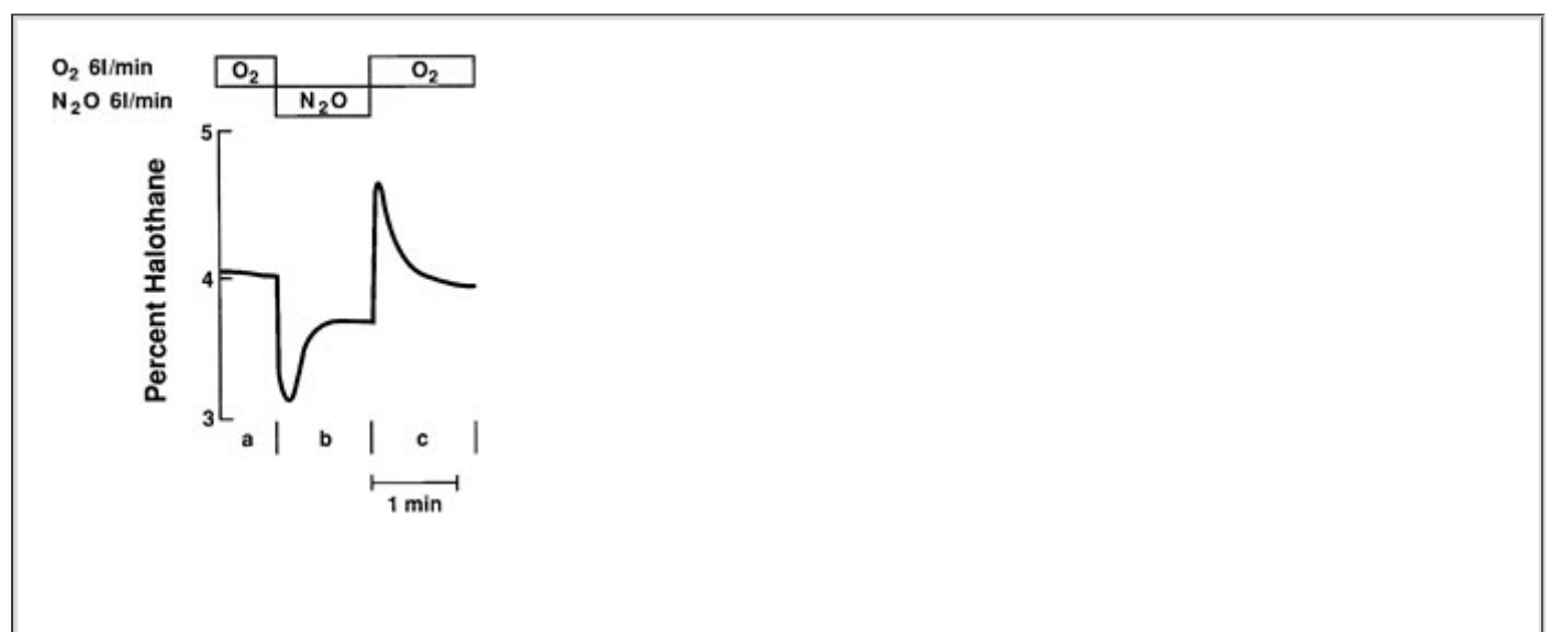
FIGURE 21-21. Halothane output of a North American Dräger Vapor 19.1 vaporizer with different carrier gases. The initial output concentration is approximately 4% halothane when oxygen is the carrier gas at flows of 6 L/min ( A ). When the carrier gas is quickly switched to 100% nitrous oxide ( B ), the halothane concentration decreases to 3% within 8 to 10 seconds. Then, a new steady-state concentration of approximately 3.5% is attained within 1 minute. See text for details. (Modified with permission from Gould DB, Lampert BA, MacKrell
