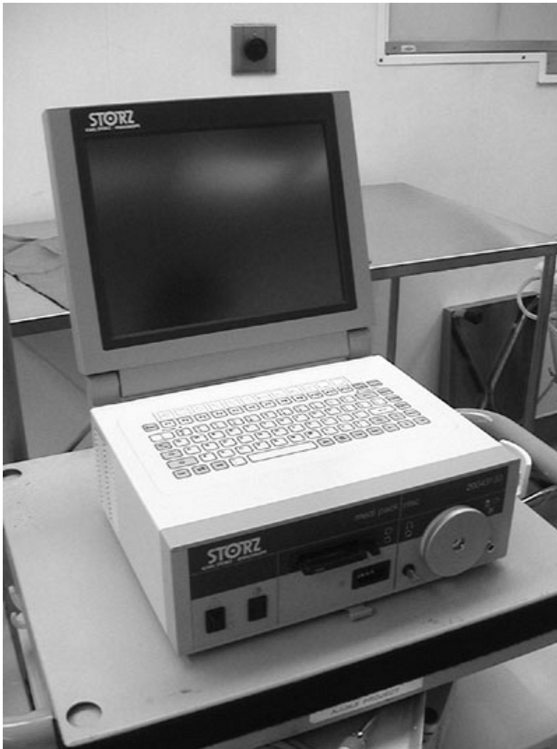
FIGURE 22-35. The Medipack (Karl Storz Endoscopy, Culver City, CA) incorporates a light source, fiberscope camera receiver, and video screen in one package.
