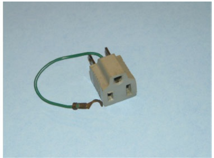
Figure 5-19 Right: a “cheater plug” that converts a three-prong power cord to a two-prong cord. Left: The wire attached to the cheater plug is rarely connected to the screw in the middle of the outlet. This totally defeats the purpose of the equipment ground wire.
