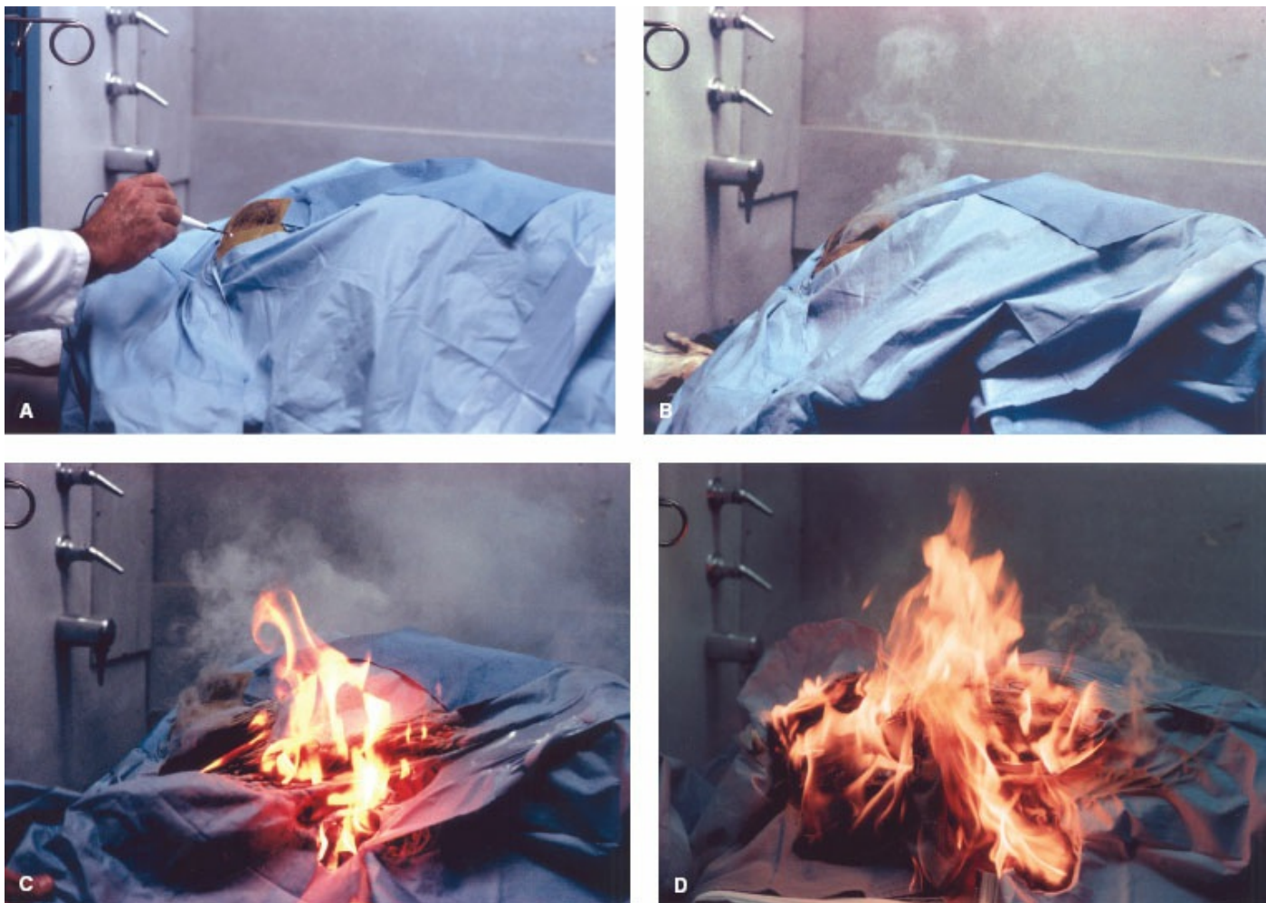
Figure 5-41 Simulation of fire caused by ESU electrode during surgery. A: Mannequin prepared and draped for surgery. Electrosurgical unit monopolar pencil electrode applied to operative site at start of surgery. B: Six seconds after electrosurgical unit application. Smoke appears from under the drapes. C: Fourteen seconds after electrosurgical unit application. Flames burst through the drapes. D: Twenty-four seconds after electrosurgical unit application. Entire patient head and drapes in flames. (Reprinted with permission from Barker SJ, Polson JS. Fire in the operating room: A case report and laboratory study. Anesth Analg. 2001;93:960. Copyright © 2001, International Anesthesia Research Society.)
