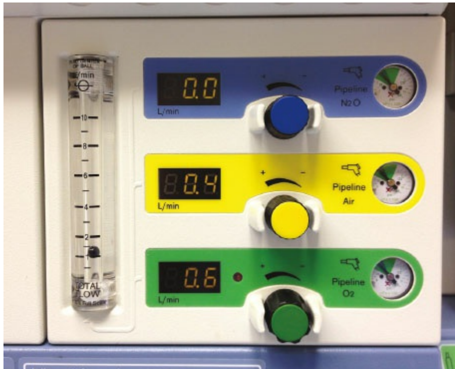
Figure 25-24 Dräger Fabius GS. Note needle valve controls, graphical and digital flow displays. The total gas flow rotameter continues to function if electrical power is lost.
