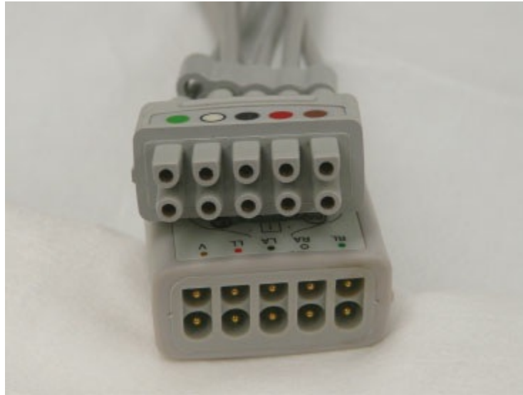
Figure 5-35 The current standard for patient lead wires ( top ) requires a female connector. The patient cable ( bottom ) has shielded connector pins that the lead wires plug into.
