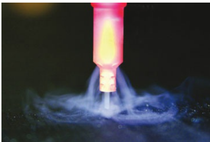
Figure 5-44 The CO 2 fire protection device with white smoke exiting the device (simulating carbon dioxide flow) and surrounding the ESU pencil tip. (Reprinted with permission from Culp WC Jr, Kimbrough BA, Luna S, et al. Operating room fire prevention: creating an electrosurgical unit fire safety device. Annals of Surgery .
