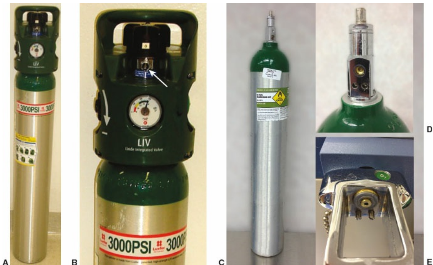
Figure 25-12 3,000 psig E-cylinder with Linde Integrated Valve, LIV (A). Linde Gas North America LLC that permits adjustable flows of ¼ to 25 L/min from the low-pressure nozzle (arrow) (B). There is also a high-pressure regulator that can supply oxygen at 50 psig via a DISS connector. Standard E-cylinder (C) showing pin-index safety system (D) and mating yoke (E).
