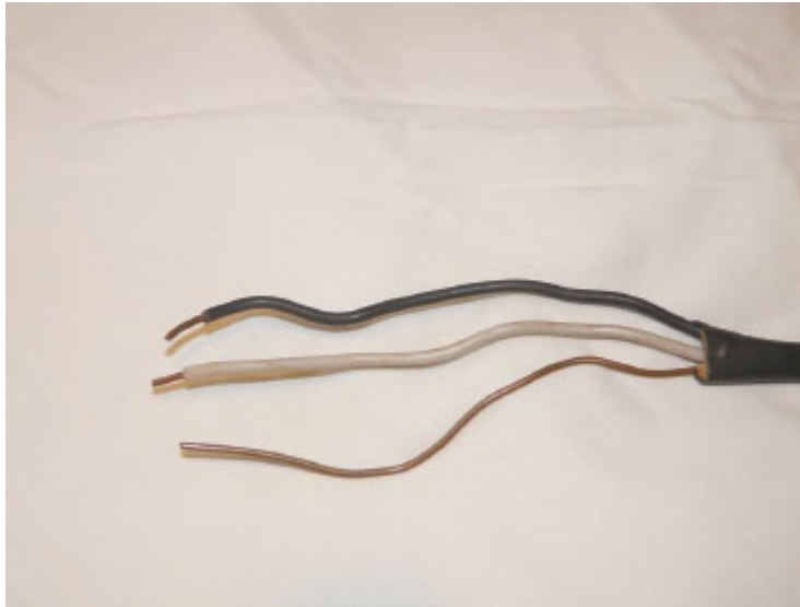
Figure 5-10 Modern electrical cable in which a third, or ground wire has been added.
