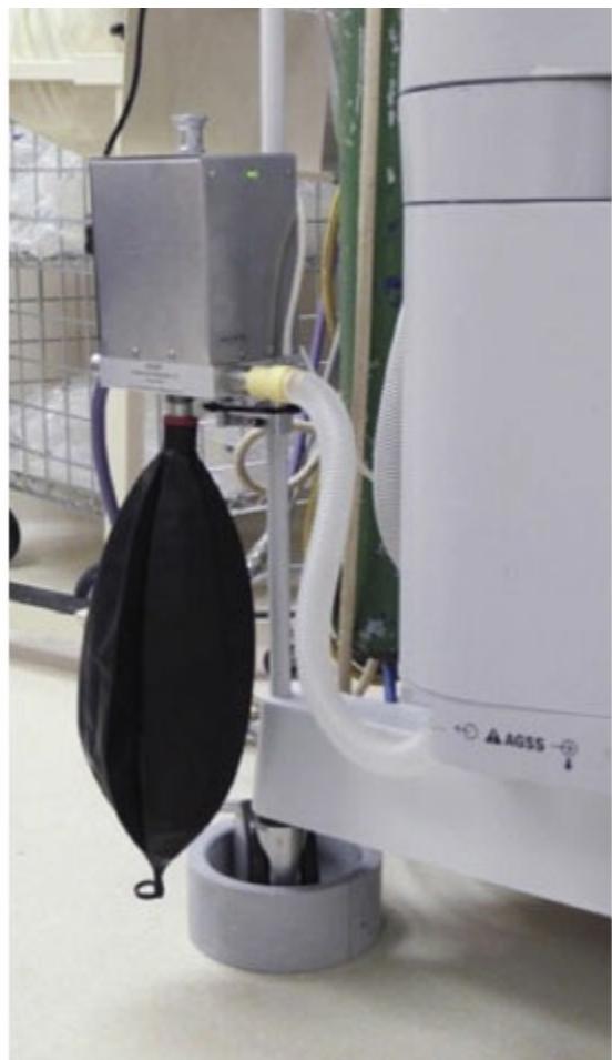
Figure 25-52 Dynamic Gas Scavenging System (DGSS). A: DGSS interface; B: Interface mounted on a GE anesthesia workstation. For details see text.
