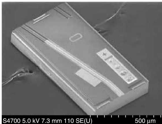
Figure 3.50 Monolithic indium phosphide-based RSOA features a curved waveguide architecture. (From Ref [82])
