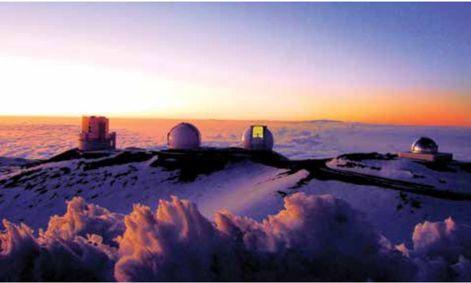
Figure 7.7 Observatories are usually located high on mountaintops, to rise above most of Earth's water vapor to improve access to the infrared portion of the spectrum. Visitors to the Mauna Kea Observatories in Hawaii have a view of the tops of the clouds, stretching away from the mountaintop.
