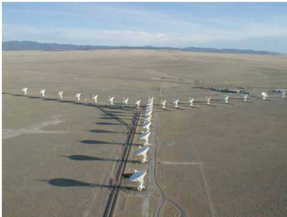
Figure 4.17 The Very Large Array (VLA) in New Mexico combines signals from 27 different telescopes so that they act as one “very large” telescope.
