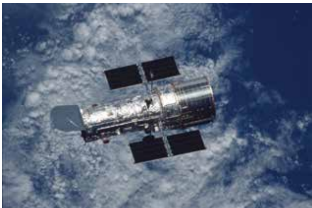
Figure 4.19 The Hubble Space Telescope observes in the ultraviolet, visible, and infrared regions of the electromagnetic spectrum.
