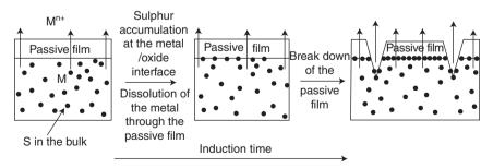
7.1 Mechanism of the breakdown of the passive film induced by enrichment of sulphur at the metal–passive film interface (Marcus, 1995). Used with permission from Taylor and Francis.
