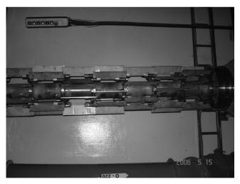
*12.2* Rotor part of a layer rotor evaporator used for increasing the salt concentration in the waste liquid and bituminisation of liquid radioactive waste.
