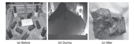
1.14 (a) In-container setup, (b) during heating, (c) resulting stable solid product.
