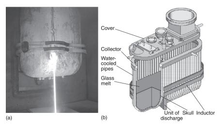
10.7 (a, b) Cold crucible for installation of liquid RAW vitrification.
