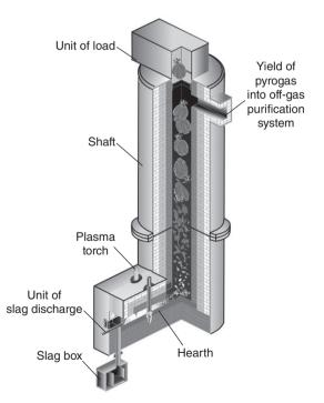
*10.8* Installation based on use of high-temperature furnace with plasma heating.
