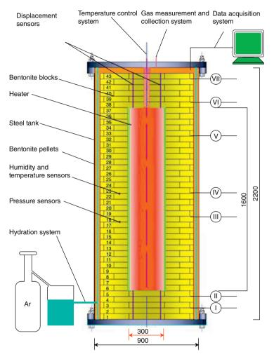
*Plate VI* (Chapter 22) Sketch of the cross-section of mock-up facility and the arrangement of central heater, steel canister, bentonite blocks/ bricks and multiple sensor arrangement.
