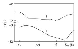
27.4 Diurnal surface temperature variation in area of thermal anomaly (Busygin and Andreev, 2004): 1, undisturbed area; 2, heat efflux area determined on photograph.
