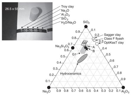
6.4 Formulation region for geopolymers compared to hydroceramics in the Na<sub>2</sub>O-SiO<sub>2</sub>-Al<sub>2</sub>O<sub>3</sub> (mol%) ternary. Note that the fourth dimension is water content and not shown on the ternary mol% diagram. The geopolymer region labeled as G1 is the target range. Optimum formulations are designated as A and B and a 1"  $\times$  2" cylindrical monolith made with composition A is shown in the photograph.
