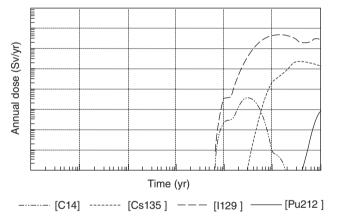
7.8 Example  $\beta$ -SOAR (Markley *et al.*, 2011) dose results for only commercial SNF using combined degradation rate in a stylized reducing geological disposal system (Ahn *et al.*, 2011a). Used with permission from American Nuclear Society (ANS).
