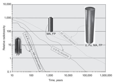
1.11 Relative radiotoxicity of SF and resulting HLW on reprocessing and recycling. FP, fission products; MA, minor actinides. The time required to achieve the initial toxicity of uranium ore is significantly reduced on recycling and transmutation of MA.
