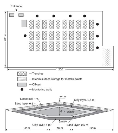
*11.4* General layout (upper figure) and separate trench cross-section (lower figure) of the 'Buriakovka' repository.
