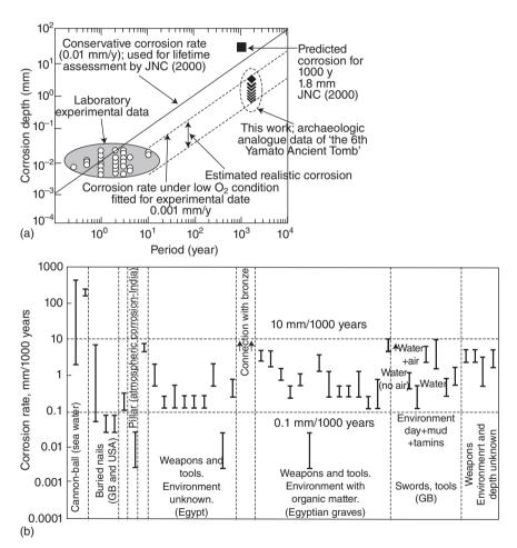
7.2 Measured corrosion rates of carbon steel in simulated solutions and correlation with archaeological analogue data up to 1,000 years: the first analysis was conducted in Japan (a) (used with permission from Elsevier), and the second in France (b) (used with permission from Maney Publishing).
