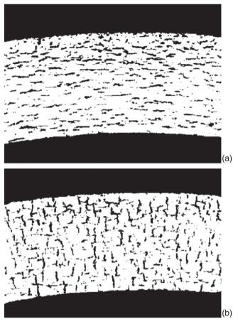
7.12 Hydride reorientation from circumferential (a) to radial (b) direction to hoop stress (Yagnik *et al.*, 2004); cladding thickness of ~0.6mm. Used with permission from American Nuclear Society (ANS).
