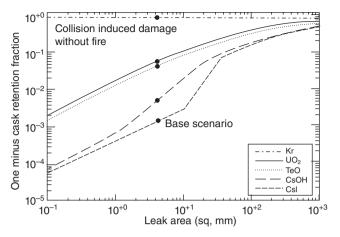
7.7 Cask-to-environment release fractions (1.0 – Retention) versus open cask surface area (Sprung *et al.*, 2000).
