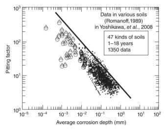
7.3 Variation of the pitting factor for carbon steel with the average depth of corrosion derived from long-term corrosion tests and short-term laboratory measurements (Johnson and King, 2008). Used with permission from Elsevier.
