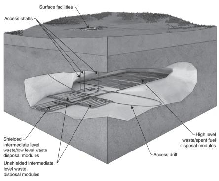
*16.10* Schematic illustration of the layout of a generic GDF (not host-rock specific) for all UK higher activity radioactive wastes. Figure courtesy of Nuclear Decommissioning Authority.
