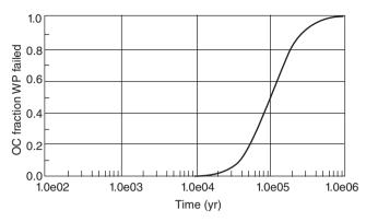
7.4 Carbon steel waste package failure time for geologic disposal system in reducing environment (Jung *et al.*, 2011). Used with permission from American Nuclear Society (ANS).
