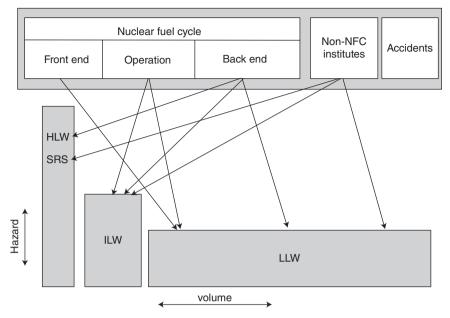
1.1 Sources of radioactive waste (adapted from Ojovan and Lee, 2005). HLW = high level waste, ILW = intermediate level waste, LLW = low level waste, SRS = sealed radioactive sources.
