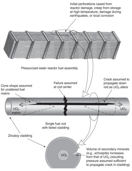
7.15 Cladding unzipping process by the oxidation/hydration of the SNF matrix or zirconium (DOE, 2002).
