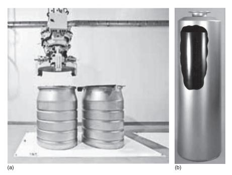
1.12 (a) 500 litre steel drums containing cemented ILW and (b) vitrified waste in 2m tall steel containers.
