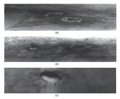
*27.1* Typical view of a thermal anomaly caused by an underground nuclear explosion on the surface during daytime (Busygin and Andreev, 2004): (a) and (b) explosion in gallery; (c) explosion in shaft.
