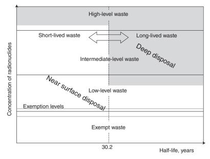
*1.20* Illustration of disposal and storage options for types of radioactive wastes.
