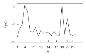
27.3 Temperature distribution on the surface measurement profile (Busygin *et al.*, 1999): the numbers N indicate the thermocouple numbers of the profile shown in Fig. 27.2.
