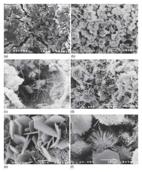
10.3 Internal chippings of cement compound core from near-surface repositories of 1960–1961 (microphotography by scanning electron microscope): (a) internal cracks; (b) friable structure, (c) pores, filled with the fibrous new formations, (d) needles of ettringite,
