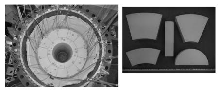
22.6 Compacted engineered bentonite blocks arranged in inside a mock-up test facility within a steel tank (top view). This mock-up THMC test consists of a heater (canister) and bentonite blocks within a cylindrical steel tank.
