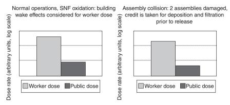
7.11 Example dose estimate for (a) oxidation and (b) collision (/drop) of SNF assemblies (after Kamas *et al.*, 2006). Used with permission from American Nuclear Society (ANS).
