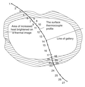
*27.2* Scheme of the thermocouple placement on a thermal anomaly (Busygin *et al.*, 1999): solid curve is the surface measurement line; the circles with numbers are the numbered thermocouples.
