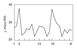
27.6 The radiation background on the surface measurement profile (Busygin and Andreev, 2004): the numbers N indicate the numbers of the thermocouples in Fig. 27.2.
