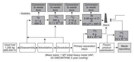
*5.5* Schematic of off-gas treatment components from a typical UNF (per kg initial U after 55 GWd/MTHM and 5 years of cooling) (Jubin *et al.*, 2009).
