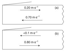
*27.5* Typical variations in the velocity and direction of the air flow in galleries (Busygin *et al.*, 1999): (a) warm period of year; (b) cold period.
