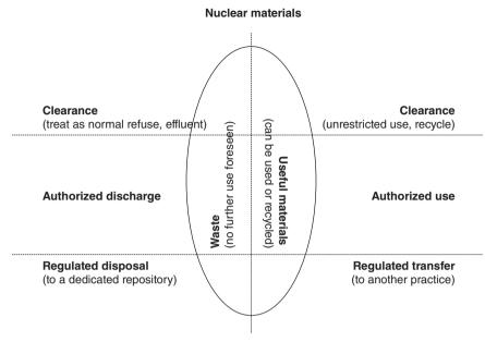
4.1 Schematic of radioactive materials routing (radioactive waste road map).
