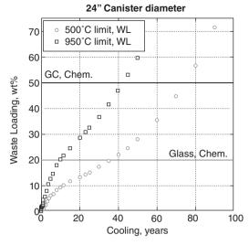
*5.6* Comparison of estimated HLW raffinate loading in glass and glass ceramic waste forms. GC, Chem and Glass, Chem represent the chemical limits for glass ceramics and glass (based on data from Crum *et al.*, 2010).
