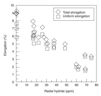
*7.13* Effects of radial hydrides on ductility (elongation) loss in a more severe case. The different orientations result in different magnitudes of ductility loss (Yagnik *et al.*, 2004). Used with permission from American Nuclear Society (ANS).
