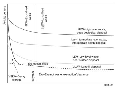
1.4 Schematic classification of radioactive wastes aiming for clearance, decay storage or disposal.
