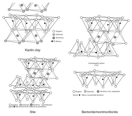
*6.2* Atomic structures of various clays (kaolin, bentonite-montmorillonite, illite). After [400, 401].
