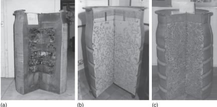
6.3 Examples of composite waste forms using encapsulation in cements where the cement physically surrounds the waste and the radionuclides may be immobilized by being incorporated into the cement phases. The ILW in (a) is compacted ILW solids, in (b) is Magnox (Mg alloy) fuel cladding swarf and in (c) is ceramic fuel zircalloy cladding hulls.
