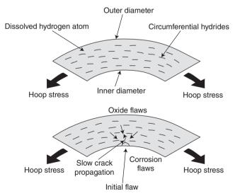
7.14 A schematic of the DHC process showing hydrogen diffusion to an existing crack tip. The threshold stress intensity factor for DHC of Zircaloy is in the range of 5 MPa m<sup>1/2</sup>. Under storage conditions, such level of stress intensification has not been demonstrated, although a few possibilities are currently under study.
