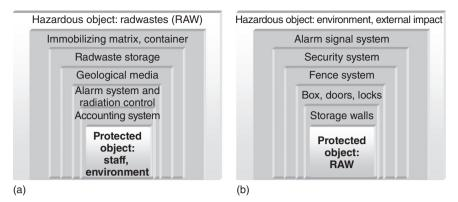
9.2 Protective shield for (a) environment and (b) radioactive waste.
