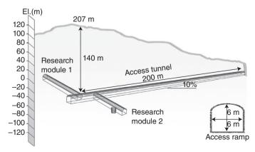
21.8 Schematic internal configuration of KURT [Cho et al., 2007].
