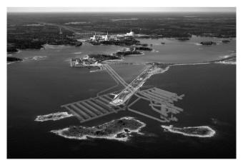
*13.2* Photomontage showing the Forsmark reactor site and the underground parts of the SFR repository in Sweden. Existing parts to the right and the planned expansion to the left (from SKB's Brochure 'SKB bygger ut SFR'. Illustrator: LAJ Illustration, Photographer: Lasse Modin).
