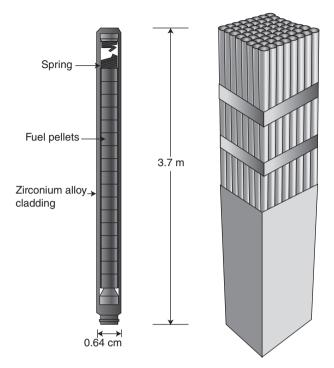
1.5 Nuclear fuel rod (left) and assembly (right).
