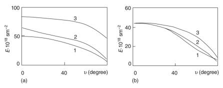
27.7 Extinction coefficient depending on sight angle for high (a) and low (b) transparency of atmosphere: 1,  $\Delta\lambda = 4-5$  micrometers; 2, 8–10 micrometers; 3, 10–12 micrometers.
