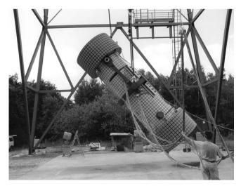
*14.3* A POLLUX<sup>®</sup> container being lifted into position for a 9m drop test. Source: Provided by the German Federal Institute for Materials Research and Testing (BAM), Berlin, Germany.
