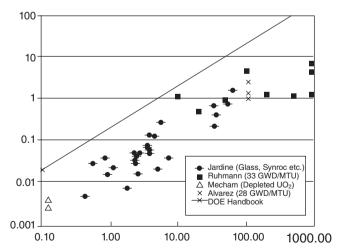
*7.10* Comparison of the DOE handbook respirable fraction equation to experimental values of the specific energy input into the brittle material (NRC, 2007).
