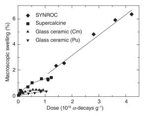
*6.6* Macroscopic swelling in Pu-doped Synroc, Cm-doped supercalcine, and Cm-doped and Pu-doped glass-ceramics. (Reprinted with permission from [166].
