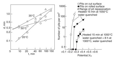
7.5 Examples of size and distribution of pits. Pit diameter vs time for 18Cr-12Ni-2Mo-Ti stainless steel in  $0.1 \text{ n} \text{ H}_2\text{SO}_4 + 0.1 \text{ n}$  NaCl. Normal pit size observed is in the range of micrometers to millimeters and pit density is for 304 stainless steel after potentiostatic polarization in 1 m NaCl solution. The term 'd' is pit diameter and 't' is time (reprinted with permission) (Szklarsksa-Smialowska, 1986). Used with permission from NACE International.
