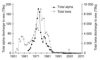
*16.9* Total alpha and total beta discharges to sea from Sellafield, 1951–2010. Note that total alpha and total beta are control measures with defined meanings under the terms of site permits.
