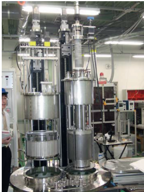
Figure 18.14 Engineering-scale electrorefiner with high-throughput anode/cathode module and the semi-continuous LCC.
