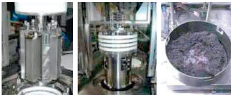
Figure 15.10 Engineering-scale electrorefiner at Toshiba (Inoue et al., 2011).
