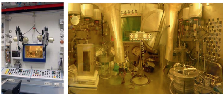
Figure 18.30 Ar-atmosphere iron-shielded hot cell dedicated to pyroprocessing studies using irradiated materials installed in JRC-ITU under collaboration with CRIEPI.
