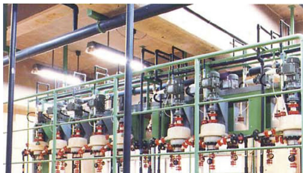
Figure 6.13 An industrial liquid-liquid extraction process using a counter cascade of Robatel BXP contactors. Photo courtesy of Rousselet Robotel ( http://www.robotel.com ).
