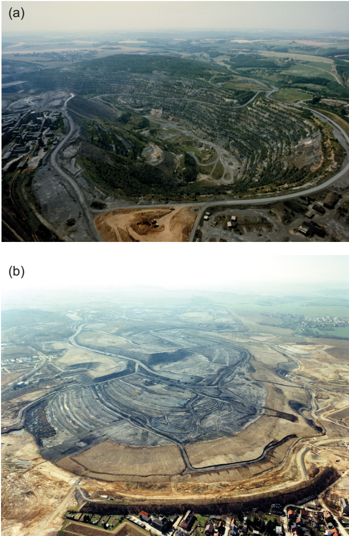
Figure 1.7 (a–c) Backfilling the open-pit mine Lichtenberg with material from various mine waste dumps. The waste material was selected such that the original geological sequence was reconstituted as far as possible.
