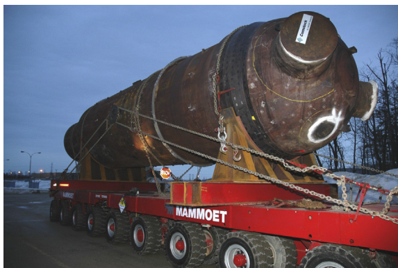
Figure 2.4 Transport of steam generator.
