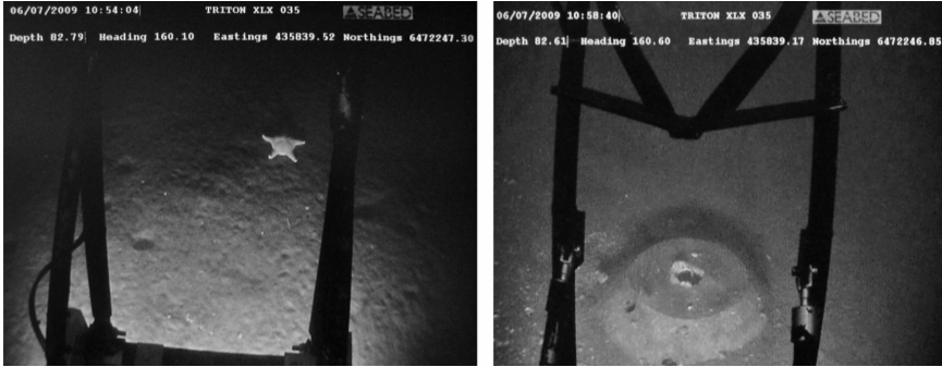
10.10 Images extracted from the ROV video, showing a starfish and one of the concrete gravimetry benchmarks on the seabed.
