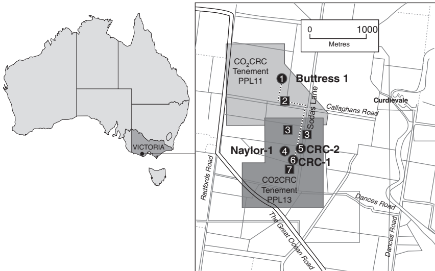
11.1 Location of the CO2CRC Otway Project in south west Victoria. The petroleum tenement boundaries are also shown. Numbered facilities are as follows. (1) Buttriss well and site of CO 2 production and compression. (2) CO 2 transport via pipeline. (3) Atmospheric, near surface and soil monitoring. (4) Naylor well used for downhole monitoring. (5) CRC-2 well used for CO 2 injection in Stage 2. (6) Visitor's Centre and control centre. (7) CRC-1 well for CO 2 injection in Stage 1.
