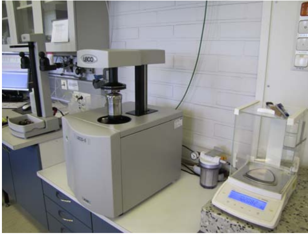
Figure 3.12 Analysis of gross calorific value with a calorimeter bomb.
