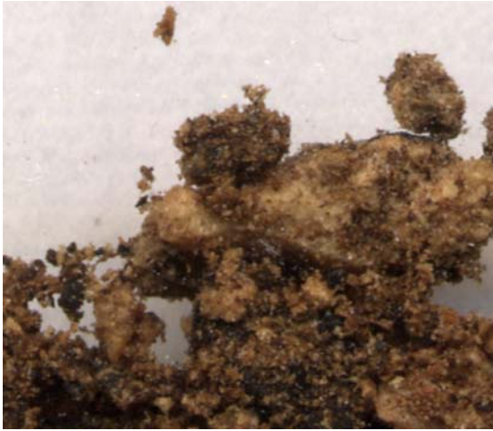
Figure 4.7 Milled palm nut kernels; a typical 'Class 2' (cohesive) biomass.
