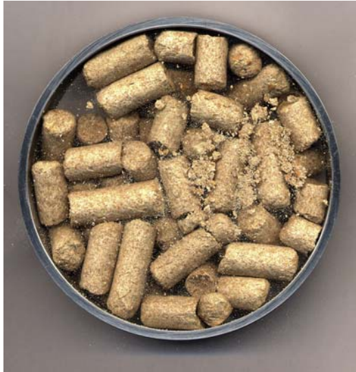
Figure 4.6 Wood pellets, a typical ‘Class 1’ (free-flowing) biomass.
