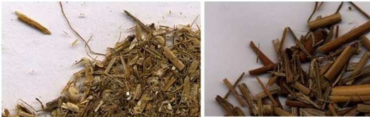
Figure 4.8 Chopped straw (left) and Miscanthus (right); typical 'Class 3' (nesting/entangling) biomass fuels.
