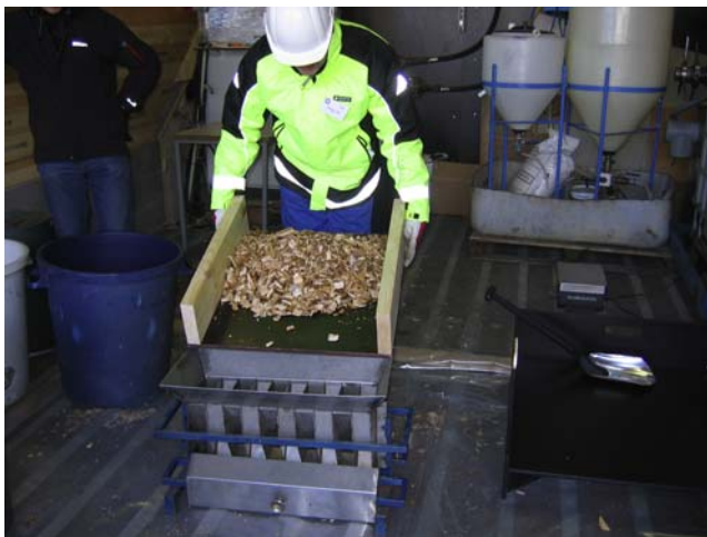
Figure 3.9 Riffle box for sample dividing.
