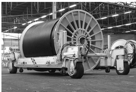
9.15 A typical high-voltage power cable made for underground installation. Drum diameter and length are approximately 3 and 4 m, respectively. Shipping weight, in this case about 60 t, and dimensions determine the maximum length of cables of a given diameter. Usually cable lengths are 700–2000 m.
