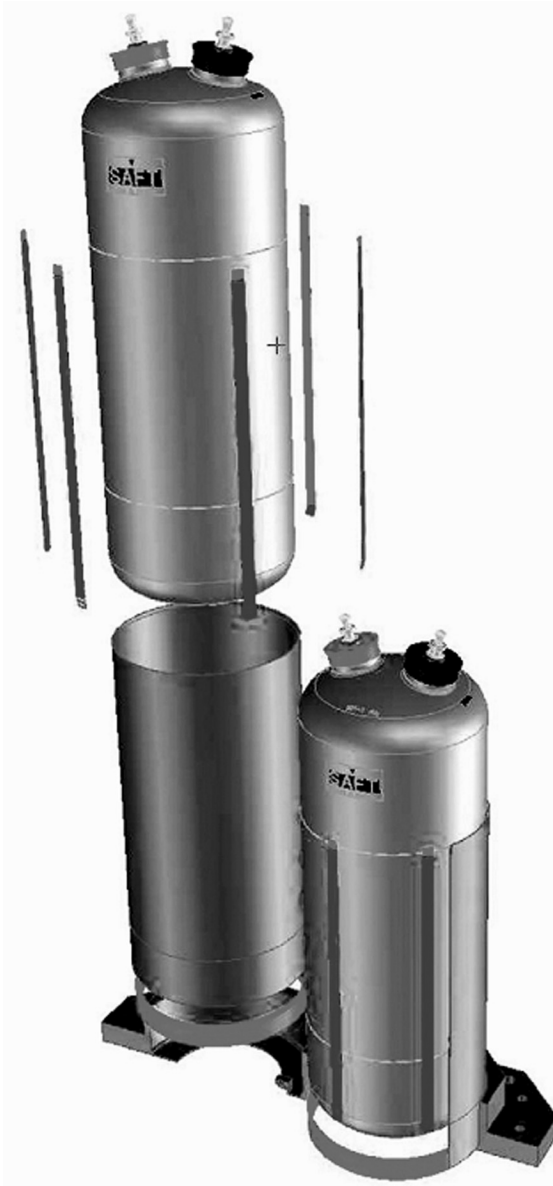
11.22 Design of SAFT Ni-H 2 battery (Borthomieu and Bernard, 2009).
