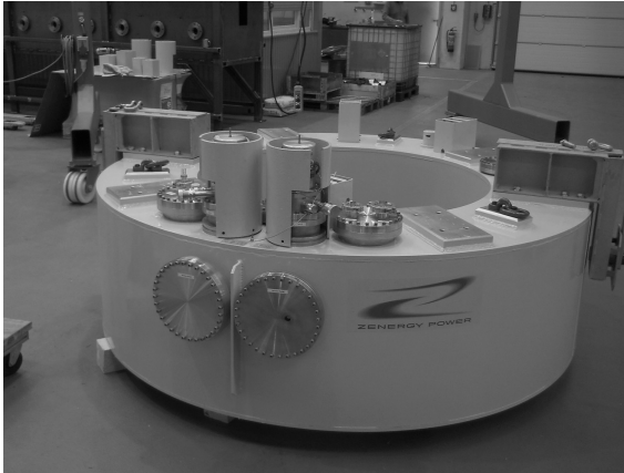
9.13 One of the two ASL/Zenergy superconducting magnets for the SFCL at CE electric. The coil uses a BSCCO-2223 from American Superconductor. It can produce a magnetic field over 2T and fully saturates the iron cores in the tank shown in the previous slide. This picture shows power leads for the coil and the flanges where two refrigerators will be installed.
