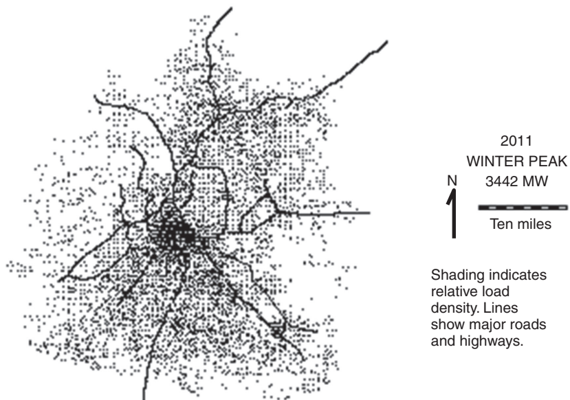
1.3 A map showing the locations of nearly 3500 MW of peak demand for a city. Only eight power stations provide power to the entire city. The T&D system’s job is to route power from those eight stations to all 385 000 energy demand sites scattered throughout the region.
