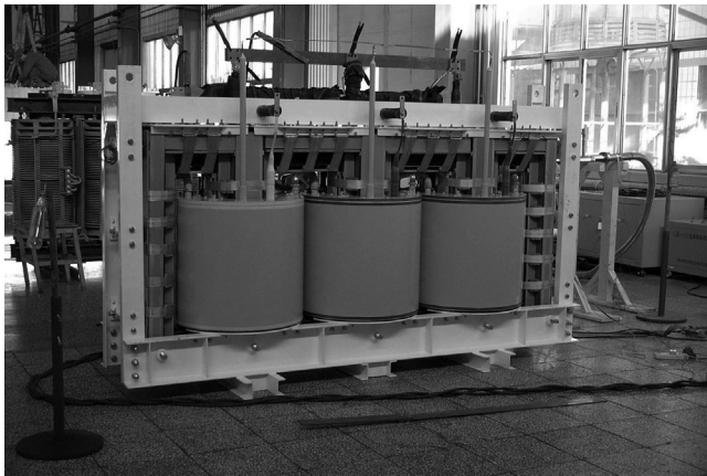
Figure 12.1 A 630 kVA HTS transformer developed by a Chinese team sponsored by the Chinese Academy of Sciences.
