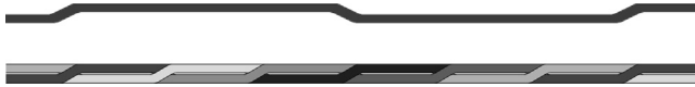
Figure 12.4 A single Roebel strand showing typical serpentine shape and six strands assembled into a Roebel cable.
