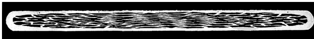
Figure 2.21 Typical multifilamentary BSCCO-2223 PIT tapes (dimension 0.3mm \times 4 mm). Courtesy of Sumitomo Electric Industries, Ltd.
