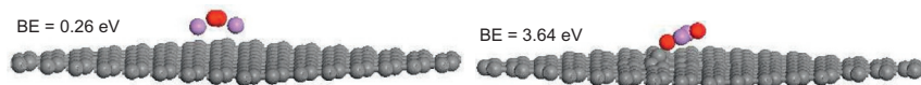
Figure 8.15 Structures of \text{Li}_2\text{O}_2 -covered pristine graphene (left) and single-vacancy graphene (right). The calculated binding energies (BE) are also given for each structure.
