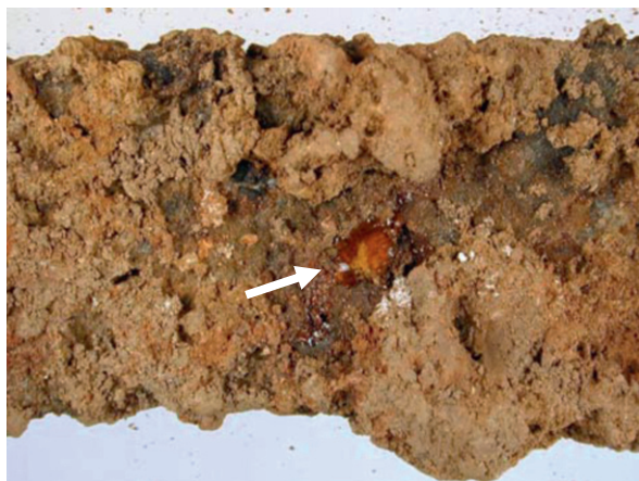
Fig. 5.4 Droplets (see arrow ) due to the presence of Fe (II) chloride, which progressively oxidizes into Fe(III) and precipitates as oxide and hydroxide
