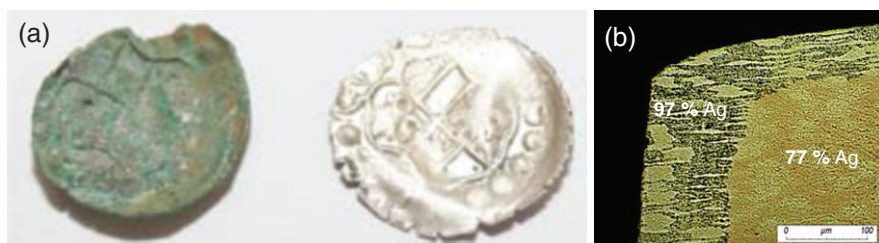
Fig. 5.12 (a) Medieval coins from the Preuschorf's hoard, as found ( left ) and after cleaning with chemicals ( right ); (b) Cross section of a test sample (80% Ag/20% Cu) showing the influence of 48 h of immersion in a cleaning solution ("silver dip") on the surface composition (after [278])
