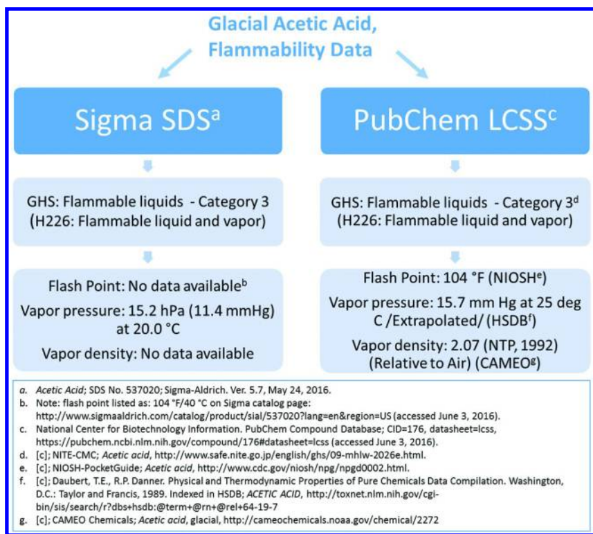
Figure 5. Flammability Data Search Process for Glacial Acetic Acid.
