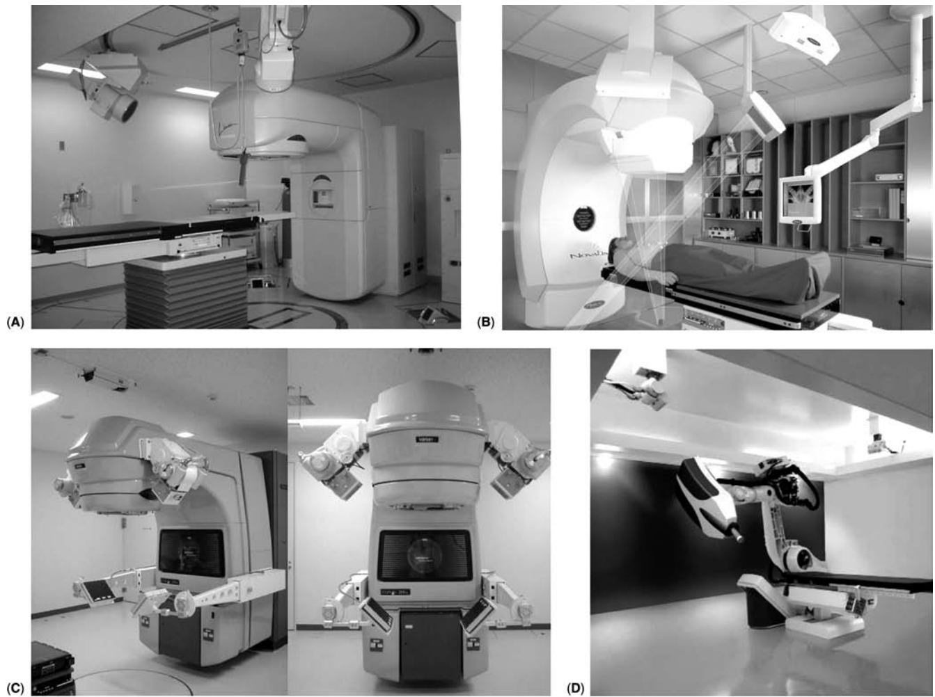
Figure 2 Real-time tumor tracking systems for RT. Three-dimensional imaging and patient positioning for high-precision dose delivery has been introduced by ceiling-mounted (A), linac gantry-mounted (B,C) and robotic systems (D). Abbreviation: RT, radiotherapy.
