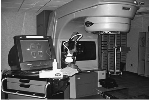
Figure 3 The BAT ultrasound in clinical practice. The ultrasound cabinet is moved adjacent to the treatment couch prior to the initiation of radiotherapy. Abbreviation: BAT, B-mode acquisition and targeting.
