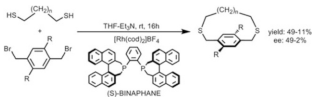
Fig. 4 Enantioselective coupling of dithiols with dibromides catalyzed by [\text{Rh}(\text{cod})_2]\text{BF}_4/(\text{S})\text{-BINAP} [73]
