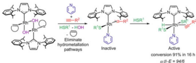
Fig. 42 Mechanism for Rh-hydroxo-NHC catalyst
