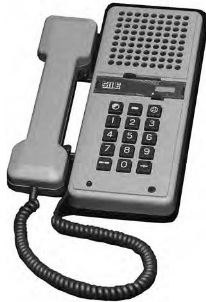
Fig. 30.18 This desktop multifunction intercom unit is usable in either handset or hands-free mode. In addition to standard intercom functions, each handset, which is connected to a central exchange, can provide additional features such as automatic redial, call conferencing, searching, all-call, group call, call transfer, call registration (stores incoming call numbers), privacy mode, special-meaning tones, and networking. The unit can also be used for voice and beeper paging. Exchanges, which can handle up to 4000 stations, are microcomputer-controlled, solid-state assemblies that vary in physical size according to the number of stations served. A typical large exchange might measure 60 in. W \times 24 in. H \times 20 in. D (1.5 \times 0.6 \times 0.5 m). (Courtesy of Dukane Corp., Communications Systems.)
