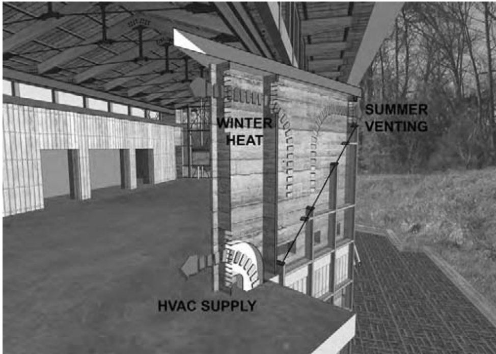
Fig. 8.64 Diagram showing integrated uses of the Trombe wall as a structural element along the exhibit space with summer venting, winter heating supply, and supplemental HVAC supply. (© Lord, Aeck & Sargent, Inc.; used with permission.)
