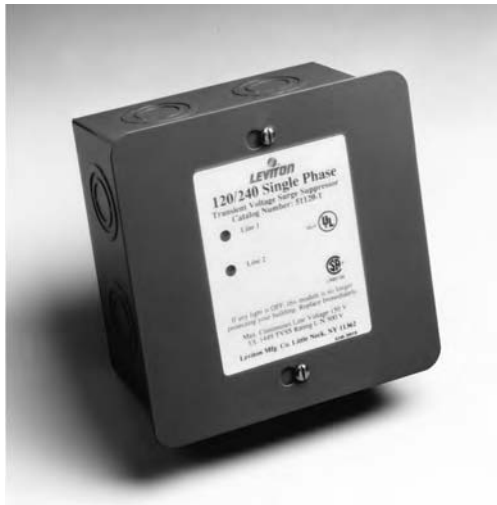
Fig. 26.61 TVSS unit designed to be used at service and branch panelboards in residences and small commercial installations. The illustrated unit is rated single-phase, 120/240 V, 3-wire service, category B3. The unit measures 7 in. W × 7 in. H × 4 in. D (180 × 180 × 100 mm) and is equipped with indicating lights that note power and suppression status. (Photo courtesy of Leviton Manufacturing Co.)
