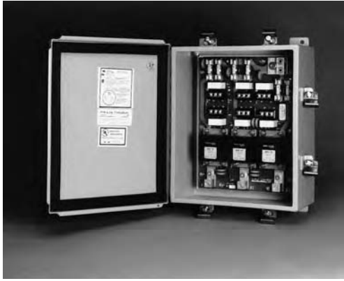
Fig. 26.60 Surge suppressor designed for use on the incoming service of a facility. It is rated for category C3 application: shunt type, 120/208 V, 3-phase, unlimited current. It is provided with RFI/EMI filtering and replaceable surge-suppressor modules, and arranged to indicate the power and protection status of each phase. (Photo courtesy of Surge Control Ltd.)
