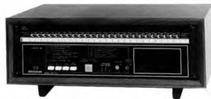
Fig. 30.14 Compact program/intercom control center. This unit, which measures 20.5 \times 11 \times 8.5 in. high (521 \times 280 \times 216 mm), has a separate power amplifier for intercom and program material. It distributes program material or provides intercom with 25 loudspeaker locations and has additional capabilities, such as emergency/all-call paging, tone calling, time signal, night bell, and telephone paging. Program material is accepted from separate external sources. (Courtesy of Bogen Communications Inc.)
