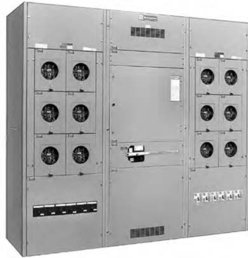
Fig. 26.7 Three-section commercial submetering switchboard comprising a center service-entrance section rated 4000-A, 3-phase, 480-V maximum, equipped (usually) with a main switch or circuit breaker. Each of the end cubicles will accept six tenant meters, each on a 320-A 3-phase circuit, maximum, protected by an integral circuit breaker or fused switch. Tenant wiring enters the top or bottom of the board. Switchboards of this type can be installed on every floor of a large multitenant commercial office building. (Photo courtesy of Cutler-Hammer.)
