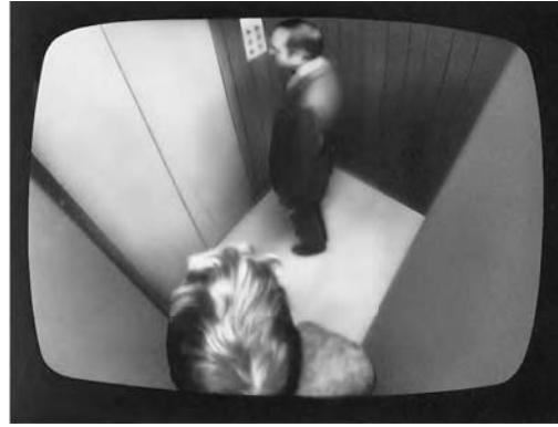
Fig. 31.34 Wide-angle TV camera intended for elevator car surveillance. A prominent printed warning in the car is an integral part of the system's effectiveness. (Photo courtesy of Visual Methods, Inc.)
