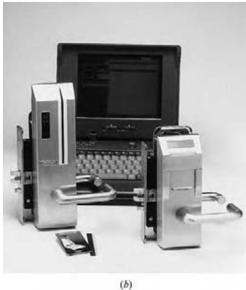
Fig. 30.25 Stand-alone electronic locking system. (a) The arrangement and interconnection of equipment at each portal are shown. The card reader (swipe or insert type) is built into the door mechanism, which also contains the electric strike mechanism. (b) Each lock (swipe style on the left and insert type on the right) is individually programmed using the laptop computer seen in the background. Each lock can be programmed for up to 1500 users, each on a time-schedule basis, covering not only working hours, holidays, weekends, and the like, but also individual time schedules. All programming is performed locally, and the passage record of each lock can be downloaded easily. (Courtesy of Ilco-Unican Corp., Electronic Access Control Div.)
