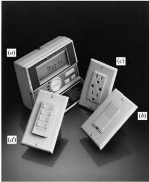
Fig. 26.57 Components of a residential-type PLC system. (a) Control unit, at which both manual and automatic (programmed) control of a maximum of 256 address codes is possible. (b) Wall-switch module has local dimming and switching functions in addition to being remotely controlled from the control center (a). (c) Duplex wall receptacle, either split-wired with local programming of one-half of the outlet or complete remote control. (d) Outlet box wall-mounted control switch that provides local group control (switching and/or dimming) for one to four devices (address codes). (Photo courtesy of Leviton Manufacturing Co.)
