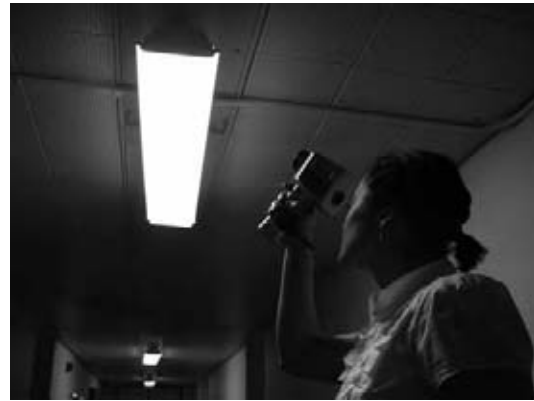
Fig. 15.11 Checking the luminance of a fluorescent fixture with a luminance meter. (Photo © 2009 by Alison Kwok; all rights reserved.)
