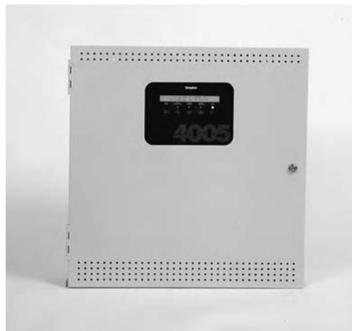
Fig. 24.62 Control panel for a hard-wired conventional system that can accommodate up to 36 detection zones. The panel has a 2-line, 80-character alphanumeric display that indicates the zone alarm, trouble signals, and diagnostics information. The panel, which is 24 in. (610 mm) square, is microprocessor controlled and field programmable. A separate annunciator can be readily connected. (Photo courtesy of Simplex.)
