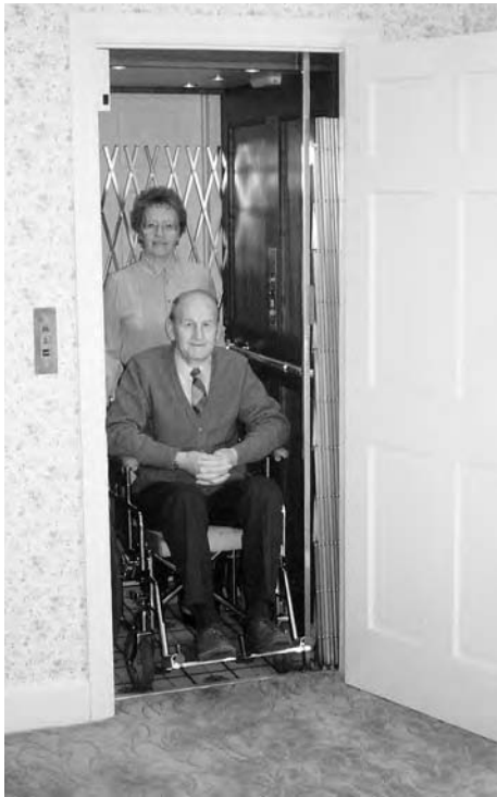
Fig. 32.14 Winding-drum residential elevator specifically designed for use by handicapped persons. The car floor area is 12 ft 2 (1.1 m 2 ), which accommodates a wheelchair plus another passenger. Note that the car is arranged with front and back access for maximum flexibility. (Courtesy of Waupaca Elevator Co., Inc.)
