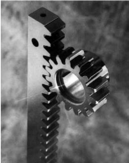
Fig. 32.11 The basis of the rack and pinion drive is simply a driven pinion on a stationary rack; rotation of the pinion forces the structure attached to the pinion to move along the rack. (Courtesy of Alimak Elevator Co.)
