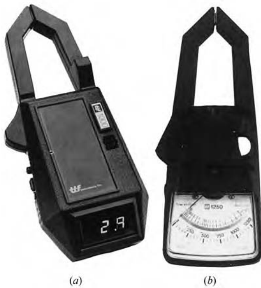
Fig. 25.18 (a) Solid-state clamp-on type meter with digital readout and automatic ranging. The latter feature eliminates the necessity to preselect a meter range and is particularly useful where the magnitude of current or voltage is unknown. The clamp-on feature permits use without wiring into, or otherwise disturbing, the circuit being measured. The meter measures approximately 8 \times 3 \times 1.5 in. ( 200 \times 75 \times 40 mm), weighs less than 1 lb (0.5 kg), and is battery-powered. Scales are 0.1–1000 amp ac, 0.1–1000 V ac, and 0.1–1000 ohms resistance, with \pm 2\% accuracy. (b) Solid-state auto-ranging clamp-on ac meter with analog-type readout. It is similar in design to the meter in (a), but with somewhat larger range scales and additional features such as peak current measurement. (Photos courtesy of TIF Instruments, Inc.)
