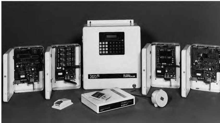
Fig. 26.17 Programmable controller (center) designed for use as an energy-monitoring and building system control device. The basic unit accepts up to 16 analog inputs, such as illuminance, temperature, kW demand load, time signals, central control signals, and the like. It processes data according to its current program (note the programming keypad) and can signal and control up to 16 outputs. Additional functions available include time-of-day switching, including astronomical considerations, and duty-cycle load switching for electric demand control. The controller is approximately 14 in. W \times 16 in. H \times 6 in. D (355 \times 410 \times 150 mm) and is arranged for surface mounting. On either side are accessory communication and relay modules. In the foreground are application software and typical sensors. (Photo courtesy of Paragon Electric Co., Inc.)
