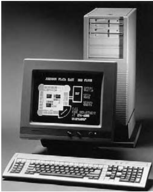
Fig. 30.31 A workstation screen shows a selected building area, its zoning, all of the area's fire/evacuation system devices and their status, and the control system's present functioning. The illustrated screen shows an active alarm condition with messages: elevators being recalled to lobby; floor is now pressurized; audio evacuation messages active; call Fire Department. (Courtesy of Johnson Controls.)
