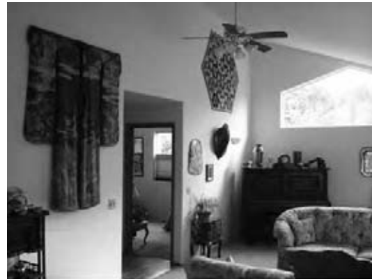
Fig. 9.4 Ceiling fans are useful in heating and cooling. In winter, at slow speeds, they destratify warm air at the ceiling. In summer (a) they extend the comfort zone by providing increased air motion. Room size is typical of residential living rooms. (Reprinted with permission of the American Society of Heating, Refrigerating and Air-Conditioning Engineers, Inc., from 1997 ASHRAE Handbook—Fundamentals.) (b) A ceiling fan is a visual feature in this Oregon residence. (Photo by Nathan Majeski.)
