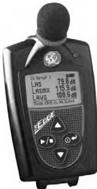
Fig. 17.20 A noise dosimeter. The unit is carried by a person whose noise exposure is being tested, with the clip-mounted microphone at shoulder (ear) level. The meter will display, store, and calculate maximum, minimum, and peak levels of SPL, Leq, TWA, exposure levels, and dosage. Noise level histories are stored and can be printed out as desired. The unit shown measures 5.5 × 2.8 × 1.4 in. (140 × 70 × 40 mm) and weighs 15.5 oz (440 g). (Photo courtesy of Quest Technologies.)
