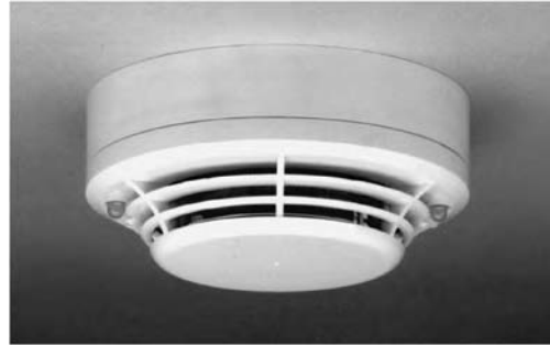
Fig. 24.48 This unit is an addressable analog laser-beam type of scattered-light photoelectric smoke detector. The sharply focused laser beam permits discrimination between smoke and dust particles, resulting in a high-sensitivity unit without false alarming. The unit is shown mounted on a sounder base containing a horn assembly, making it applicable to small, enclosed rooms. (Photo courtesy of Notifier, division of Pittway.)
