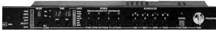
Fig. 30.12 User-programmable master clock and program controller. This unit has nonvolatile memory, eight program zones, automatic daylight saving time and holiday adjustment, and a maximum of four schedules; it is usable with most types of secondary clocks. (Courtesy of Rauland-Borg.)
