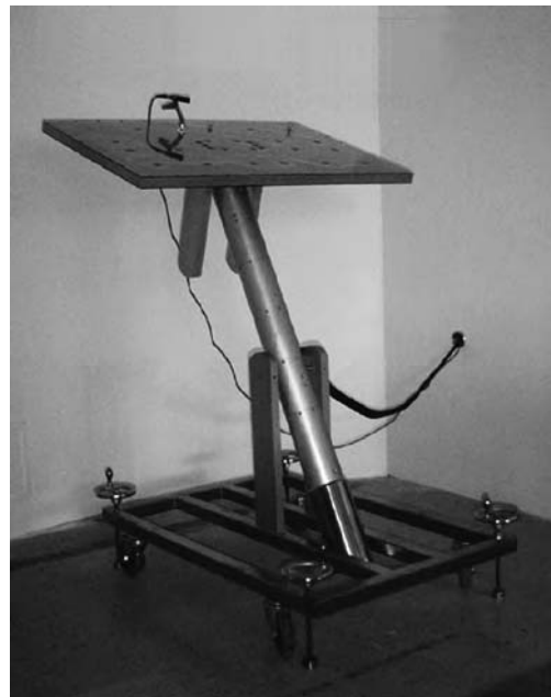
Fig. 14.40 ShadowTracker heliodon at the Baker Lighting Lab at the University of Oregon. Automated adjustments for latitude, elevation, and tilt permit exposure of the model to desired clear sky conditions. (Photo by Sara Goenner; © 2004 Alison Kwok; all rights reserved.)
