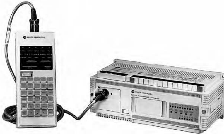
Fig. 26.18 General-purpose programmable controller. The processor unit contains the central processing unit (CPU), random access memory (RAM), and power supply. Peripherals include the illustrated hand-held programming unit and EEPROM (electrically erasable programmable read-only memory) module, and various computer/software interfaces (not shown). The unit illustrated, which measures approximately 10 \times 9 \times 3 in. ( 255 \times 230 \times 75 mm), has 16 input/output (I/O) circuits and an 885-word memory. It is readily adaptable to a variety of automated control processes in manufacturing, building control, and material handling. (Courtesy of Allen-Bradley Co.)
