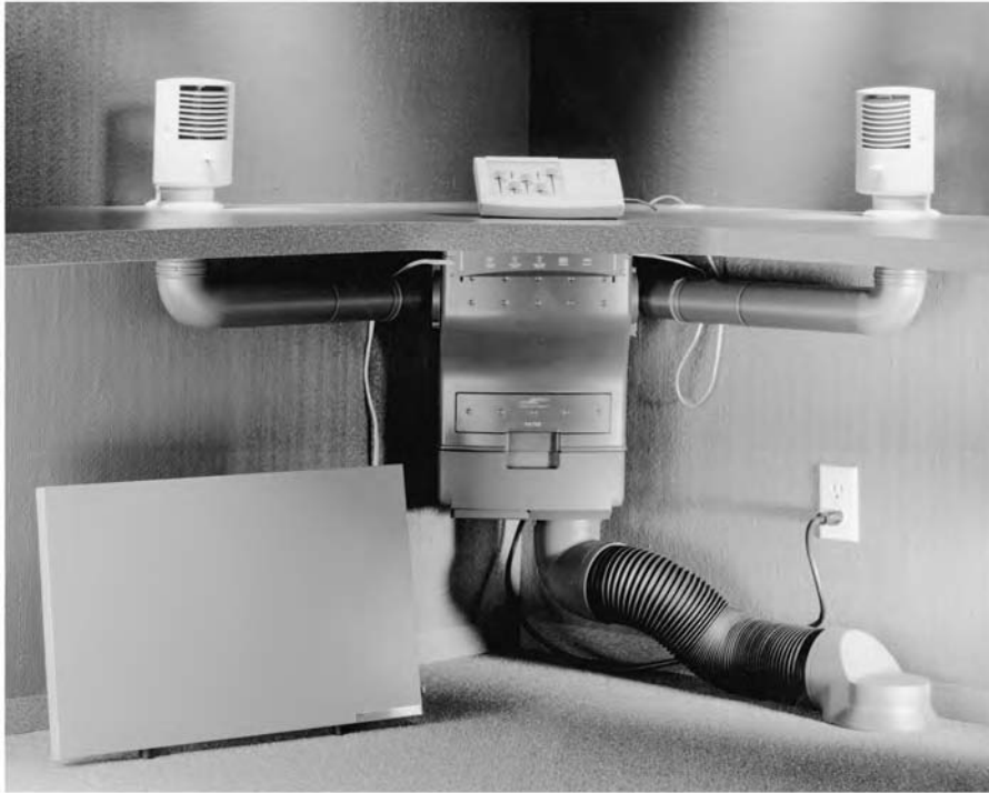
Fig. 10.49 The Personal Environments ® system provides each workstation with a fan, air filters, an air-mixing box, and a background sound (white noise) generator. The control panel allows adjustment of task lighting, background sound, fan speed, primary/recirculated air mixture, and radiant heating. Two diffusers distribute both air and background sound. Diffusers are adjustable about both horizontal and vertical axes. The below-desk radiant heating panel warms the lower body. (Courtesy of Johnson Controls, Inc., Milwaukee, WI.)
