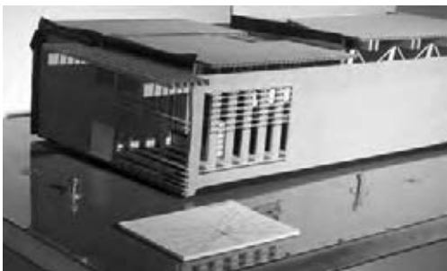
Fig. 6.10 A sunpeg chart attached to the base of a scale model to study solar access and shadow patterns in and about a building. (Photo by Jonathan Meendering; © 2004 Alison Kwok; all rights reserved.)
