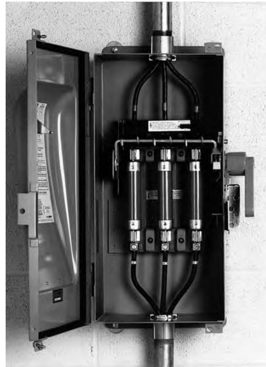
Fig. 26.10 The internal construction of a heavy-duty, fused, 3-pole, 3-wire switch in an industrial NEMA 12 enclosure. Note the gasketing on the inside of the cover, which seals the sheet steel box and makes it usable in environments containing lint, dust, dirt, sawdust, and the like. The external handle is a double-lockable indicating type for safety. (Courtesy of Siemens Energy & Automation, Inc.)
