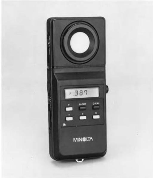
Fig. 11.48 A hand-held lightweight ( \approx 8 oz [225 g]) chromaticity meter for determining the chromaticity and color temperature of a light source. The unit reads X and Y coordinates, color temperature in degrees Kelvin, and illuminance in lux. (Courtesy of Minolta Corp.)
