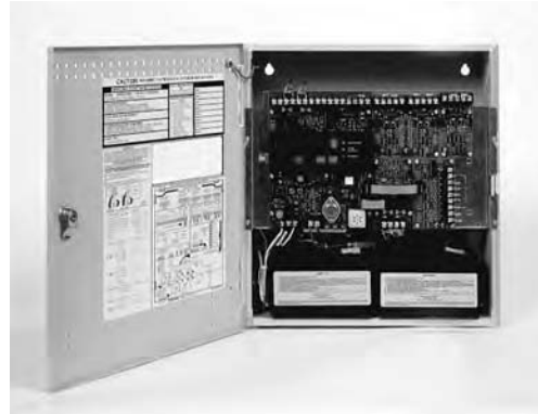
Fig. 24.61 Conventional hard-wired eight-zone (maximum) solid-state fire alarm control panel for supervised Class A or Class B circuits. A single annunciator light indicates the alarmed zone. Alarm verification for each zone is provided. Both audible and visible alarms can be used on two alarm-signal circuits. The audible evacuation signal is a slow (20-BPM [beats per minute]) or fast (120-BPM) march time. Note the two standby batteries at the bottom of the cabinet. The unit measures approximately 16 in. (400 mm) wide and 17 in. (432 mm) high and is designed for surface mounting on 16-in. (400-mm) o.c. studs. (Photo courtesy of Simplex.)
