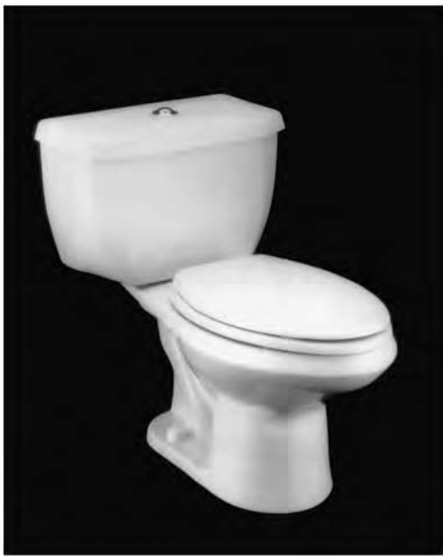
Fig. 21.46 Example of a 1.5-gal-flush (5.7-L), pressure-assisted, direct-fed siphon jet flush action flushometer tank, with a large 10 × 12-in. (250 × 300-mm) water surface area in the bowl: the Cadet Aquameter. (Courtesy of American Standard, Inc., Piscataway, NJ.)
