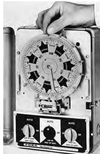
Fig. 26.13 Time switch arranged for three different types of control functions that are applicable to different types of load: (1) full photocell control—security lighting; (2) dusk “On,” preset “Off”—signs, parking lots; (3) preset on, off—interiors. This unit’s dial is a 7-day calendar type that permits setting a different schedule for every day of the week. The dial is not astronomical (solar) because all the turn-on functions are either photocell or time-of-day controlled. Solar dials are useful when photocell control is not used because sunrise and sunset times vary with the season. (Courtesy of Tork, Inc.)
