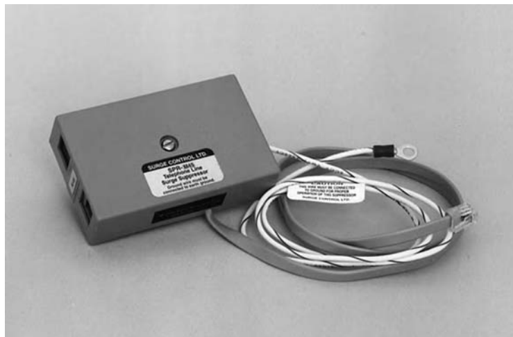
Fig. 26.64 Surge suppressor designed for use with standard snap-in low-voltage telephone and industry jacks. The illustrated unit is designed to protect telephone/telecommunication lines, both analog and digital. The units are rated 185 V, with a maximum surge current of 5000 A and a test clamping voltage of 240 V. The units can be used with telephones, modems, fax machines, and the like. They measure approximately 4 in. W \times 2½ in. H \times 1 in. D (100 \times 64 \times 25 mm). (Photo courtesy of Surge Control Ltd.)
