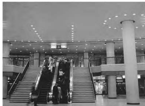
Fig. 13.20 The lines of light fixtures in the center converge optically to produce a directional flow of traffic toward the escalator. (Penn Station, New York; photo by B. Stein.)
