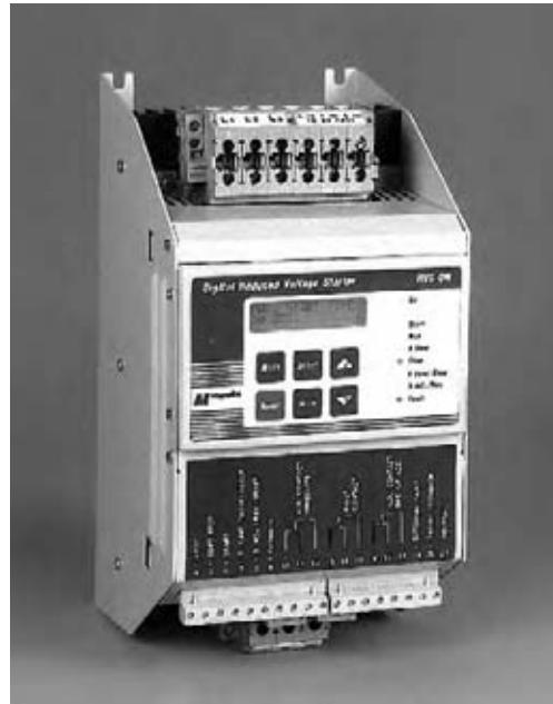
Fig. 26.37 Soft starter type for 3-phase induction motors of up to 1400 hp (1045 kW), shown without an enclosure. This microprocessor-based unit provides two selectable starting characteristics with stepless acceleration, plus additional control and protection functions including reversing control, over- and undervoltage and current protection, and two normal motor operating speeds. (Photo courtesy of Magnetek.)
