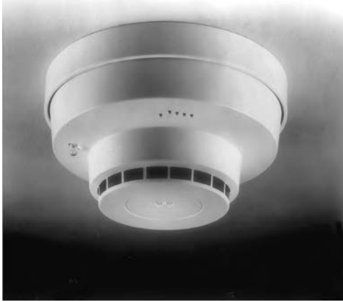
Fig. 24.46 Addressable analog (intelligent) scattered-light-type photoelectric smoke detector with an on-board microprocessor that negates false-alarm signals caused by radio frequency and electromagnetic interference (RFI/EMI). It also validates trouble signals. If required, this unit can be equipped with a resettable heat detection element. The unit is approximately 5½ in. (140 mm) deep and 3 in. (75 mm) high. (Photo courtesy of Cerberus Pyrotronics.)
