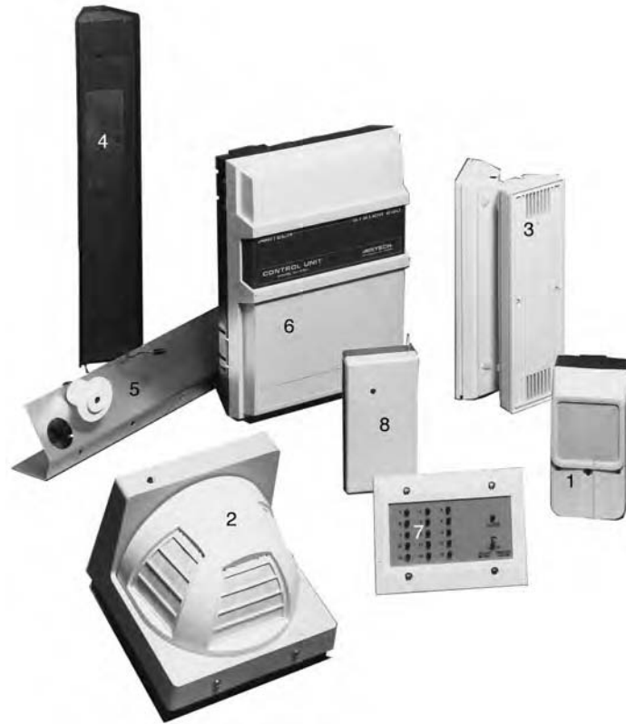
Fig. 30.2 Typical intrusion detection equipment: (1) Passive infrared detector. Maximum sensitivity is a 4^{\circ}\text{F} ( 2^{\circ}\text{C} ) differential between target and background and a target motion of 2\frac{1}{2} in./s (64 mm/s). The unit is approximately 6 in. (150 mm) deep. These detectors are available with different coverage patterns and a maximum coverage of 2000\text{ ft}^2 ( 185\text{ m}^2 ). (2) High-sensitivity, multizone, wide-angle passive infrared detector gives coverage of 17 zones horizontally and vertically. (3) Ultrasonic detectors arranged to give broad coverage of approximately 200 \times 50\text{ ft} ( 61 \times 15\text{ m} ). Each unit is 11 \times 5\frac{1}{2} \times 3\frac{1}{2} in ( 280 \times 140 \times 90\text{ mm} ). (4) High-sensitivity, balanced signal type of ultrasonic detector differentiates between an intrusion signal and random environmental signals, thus reducing false alarms. (5) Unobtrusive, button-type ultrasonic sensor intended for ceiling mounting. (6–8) System control panel, annunciator, and mechanical alarm interface units. (Photos courtesy of Sentrol, an SLC Technologies Company.)
