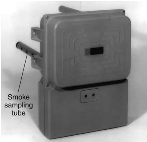
Fig. 24.47 This smoke detector, intended for duct mounting, can utilize either a photoelectric or ionization-type head. The unit, which is usually mounted in return-air ducts rather than supply ducts to minimize smoke dilution effects, uses an air-sampling tube that extends across the full width of the duct. Duct smoke detectors are intended primarily to prevent smoke dispersal throughout a building by causing shutdown of the air-handling system and by control of smoke damper operation. (Courtesy of Simplex.)
