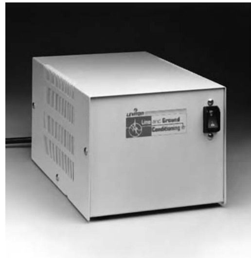
Fig. 26.58 This single-phase power conditioner supplies noise filtering and surge suppression by use of an isolation transformer, ground noise filters, and category A and B surge suppression (see Section 26.37c). It is rated 5 A, 120 V, measures 6 in. H × 7 in. W × 11 in. D (150 × 180 × 280 mm), and weighs 18 lb (8 kg). A similar unit rated 20 A, 120 V measures 8 in. H × 8½ in. W × 14 in. D (200 × 215 × 355 mm). (Photo courtesy of Leviton Manufacturing Co.)
