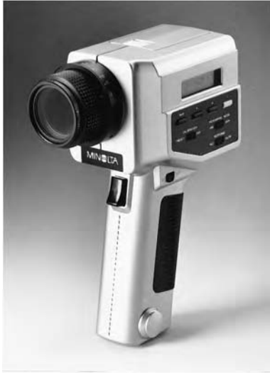
Fig. 11.10 Direct-reading, narrow-angle, spot-type luminance meter has an acceptance angle of 1^\circ , a range of 0.001 to 299,000 \text{cd}/\text{m}^2 ( 0.001 to 87000 fL), a variable response speed to permit measurement of flickering sources, and a comparison mode that permits direct luminance comparison of two sources. Results are displayed digitally. (Courtesy of Minolta Corp.)
