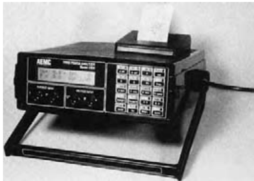
Fig. 25.23 This portable, programmable power analyzer unit measures approximately 13 × 7 × 12 in. (330 × 180 × 305 mm) and weighs 6 lb (2.7 kg). It is capable of measuring (and computing) 19 electrical parameters, among which are current, voltage, energy, power, power factor, and frequency, and of providing both an instantaneous digital readout and printed records (hard copy). Connections permit all functions to be addressed by remote control. (Courtesy of AEMC Corporation.)
