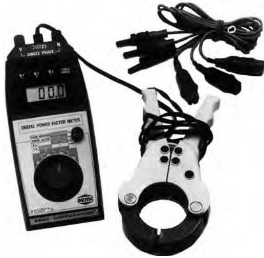
Fig. 25.22 Digital power factor meter, which measures the power factor on single- and 3-phase circuits. In addition, the meter can measure 0–600 V ac and 0–2000 A ac. Connections to the circuits being measured are made with the clamp-on probes shown. A similar unit is available that measures power in both sinusoidal and nonsinusoidal waveforms in the range 0.1 W through 2000 kW. (Courtesy of AEMC Corporation.)
