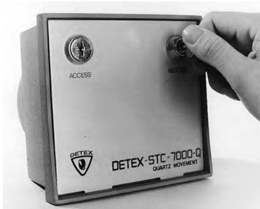
Fig. 30.17 Watchman's tour station. Here the clock and recording tape are inside. The station is operated by simply inserting a key, as shown, and giving it a quarter-turn. An alternative version of this system, commonly used, consists of a portable clock and tape operated by a key in a wall box at each station. (Courtesy of Detex Corp.)
