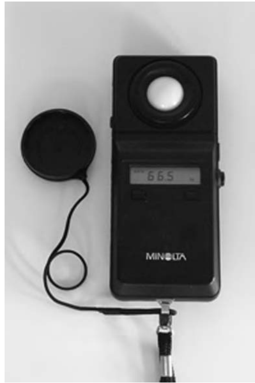
Fig. 11.8 Electronic, digital, color-corrected and cosine-corrected light (illuminance) meter from Minolta. (Photo by Jonathan Meendering.)
