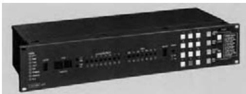
Fig. 30.13 Intercom controller. The illustrated microcomputer design interfaces with the existing telephone system. In addition, it provides paging, tone distribution, and program distribution, with control from a telephone. The unit, which measures 19 in. \times 9.5 in. \times 3.4 in. high (483 \times 241 \times 86 mm), weighs 9 lb (4 kg), also has a built-in master clock. (Courtesy of Rauland-Borg.)
