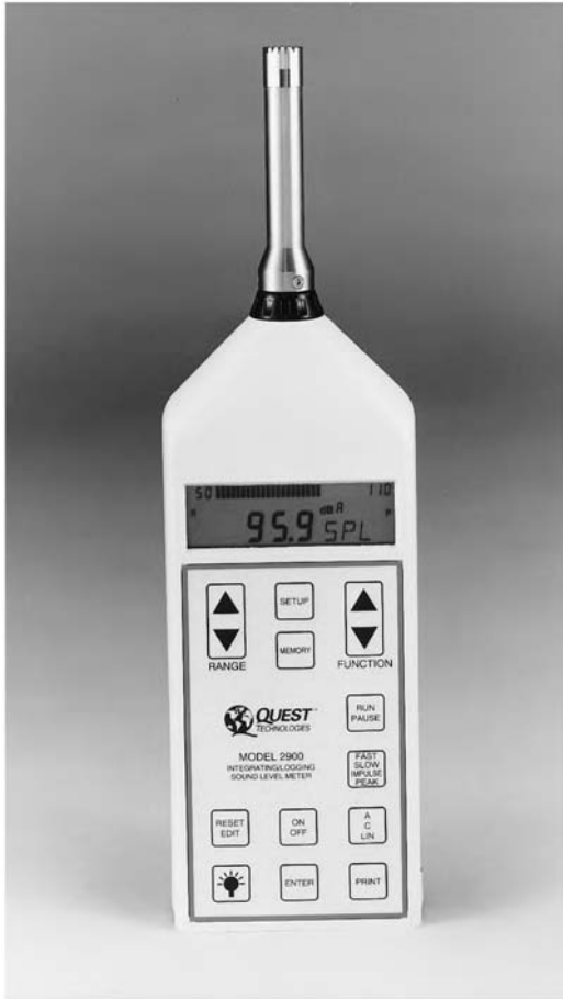
Fig. 17.15 Modern general-purpose (type 2) integrating, data-logging sound level meter. This unit will measure and record isolated, nonrepetitive noise events in addition to continuous, fluctuating, and impulsive sounds, and will give both instantaneous and equivalent (Leq) sound levels. The latter are used when an equivalent noise level of varying sound conditions over a selected measurement time is required. The meter will measure dBA, dBC, and linear with fast, slow, peak, or impulse response. When equipped with a filter set, the meter can be used for octave or 1/3-octave analysis. (Photo courtesy of Quest Technologies, Inc.)
