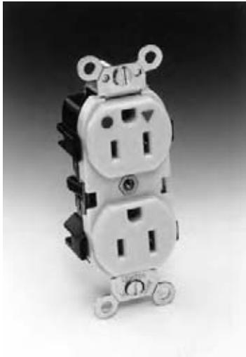
Fig. 26.45 Hospital-grade, insulated (isolated) ground receptacle used where heavy duty is expected, and both reliability and freedom from electronic noise are required. Hospital grade is denoted by a green dot on the upper left of the receptacle face, and the insulated ground by an orange triangle on the upper right. (Some manufacturers make the entire receptacle orange.) (Photo courtesy of Leviton Manufacturing Co.)
