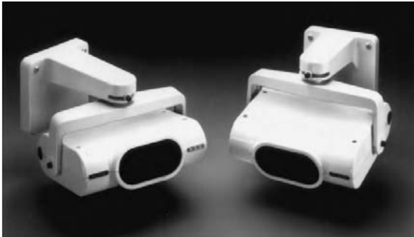
Fig. 24.43 This projected beam smoke detector utilizes an infrared (IR) beam so that ambient light will not affect its operation. Two sensitivity levels are available that are selected to match the distance between transmitter and receiver. Because heat attenuates or deflects the IR beam, the receiver translates this beam strength reduction as obscuration, identical to smoke obscuration. This effect makes the IR projected beam detector sensitive to high-heat flaming fires as well as smoky smoldering ones. (Photo courtesy of Notifier, division of Pittway.)
