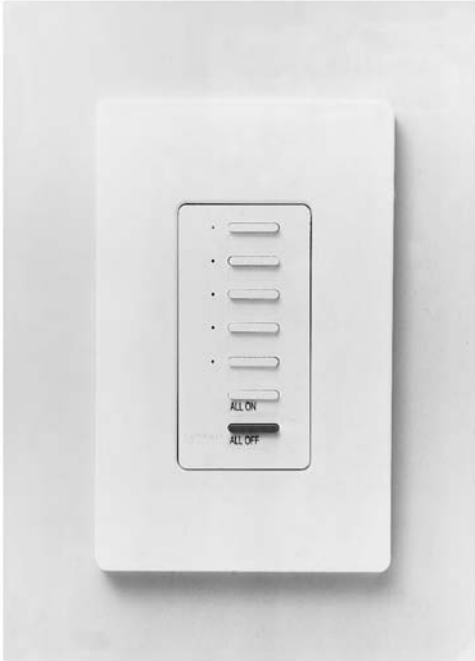
Fig. 16.5 Typical wall-mounted master station has five control buttons in addition to “All On” and “All Off” on every master. The control buttons can be arranged to control a single outlet or a group to establish lighting of a scene. Thus, the entry unit might have homecoming, extended absence, pathlighting, nightlighting, and garage-lighting scenes, whereas the kitchen master may have lighting scenes for breakfast, dinner, formal and informal entertaining, and night. Each scene can be arranged to turn on, brighten or dim, and shut off selected lighting. (Courtesy of Lutron Electronics Co., Inc.)
