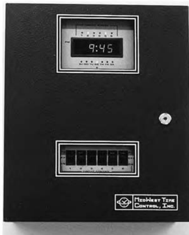
Fig. 30.11 Typical microprocessor-based master time clock and program device. This unit, which measures 14 × 12 × 5 in. deep (355 × 305 × 127 mm), provides time correction signals to synchronous wired clocks of the digital or analog type, and can be adapted to control minute impulse clocks. Programming of output circuits can be daily or weekly, and can accommodate daylight saving, holiday, and leap-year updates with a total program capacity in excess of 600 events. Programming is done locally or via a remote computer. This type of device is applicable to any facility requiring a clock and/or program system. (Courtesy of Midwest Time Control Inc.)
