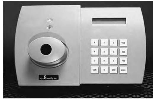
Fig. 30.26 This foolproof identification procedure relies on the fact that no two persons have identical retinal vascular patterns. The illustrated device, usually placed at an unmanned controlled-access portal, scans the entrant's retina, compares it to a previously recorded pattern, and then either permits or denies entry. (Photo courtesy of Eyedentify Inc.)
