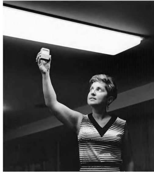
Fig. 11.11 When the cell of a direct-reading illuminance meter is held in contact with a luminous source, the surface luminance can be read directly or simply calculated.
