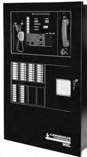
Fig. 24.65 A multiplex emergency voice alarm/communication system panel used in large high-rise buildings in conjunction with the fire alarm system panel (Fig. 24.64). The panel controls and feeds a multiplexed voice alarm system, as well as strobe light circuits and a complete firefighter's telephone intercom. It provides evacuation, alert, page, and auxiliary signals to all building speakers selectively. An integral annunciator indicates which audio devices are connected to which of the three available audio channels. All audio risers are fully supervised and power limited. (Photo courtesy of Cerberus Pyrotronics.)
