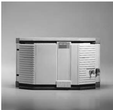
Fig. 30.39 A unitary controller is designed to control single-zone HVAC subsystems such as heat pumps, fan-coils, and the like. It is preset from the network level but can also be locally monitored and adjusted to satisfy local requirements. These adjustments are made with a portable plug-in control unit. (Courtesy of Johnson Controls.)
