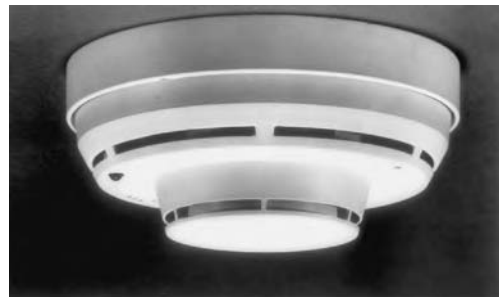
Fig. 24.41 Addressable analog (intelligent) ionization-type smoke detector with an integral microprocessor that operates the unit's detection, diagnostic, and error-checking procedures. The detector is self-adjusting to compensate for sensitivity changes due to environmental conditions. Operating sensitivity is remotely adjustable from the control panel. (Photo courtesy of Cerberus Pyrotechnics.)
