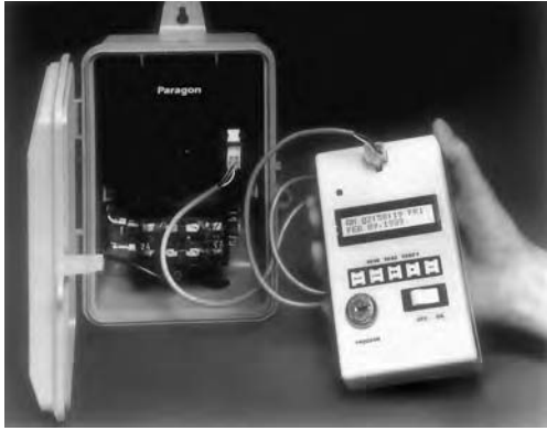
Fig. 25.14 Programmable electronic time control switch designed for time-of-use (off-peak) utility rate schedules. The programming device is separate from the switch and can be used by a utility to program many customer switches. The illustrated unit is arranged for 365-day scheduling, which permits full coordination with utility schedules that vary with the seasons of the year. Typical controlled loads include water heaters, thermal storage units, water and air accumulators, and any other load that either inherently or by design can be delayed for several hours. (Courtesy of Paragon Electric Co., Inc.)
