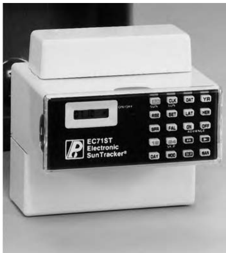
Fig. 26.15 This unit controls two 15-A, 240-V circuits. The built-in astronomical feature automatically adjusts the on-off setpoint according to sunset and sunrise throughout the year. (Courtesy of Paragon Electric Co., Inc.)
