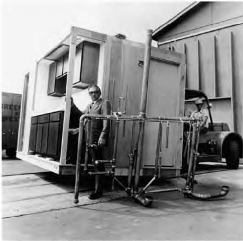
Fig. 22.25 Preassembled plumbing tree for manufactured housing, along with the prefabricated kitchen/bath in which it is installed. (Courtesy of Wausau Homes, Inc., and the Copper Development Association.)
