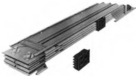
Fig. 27.10 Construction of one type of plug-in busduct. Plug-ins are evenly spaced on alternate sides to facilitate connection of plug-in breakers, switches, transformers, or cable taps. Housing is of sheet steel with openings for ventilation. The cover plate is not shown. (Courtesy of Square D Company.)
