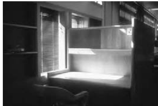
Fig. 14.6 (a) Windows adjacent to a wall provide an additional reflecting surface. (b) Reading carrel adjacent to a window at the Graduate Theological Union Library, Berkeley, California. (Drawing by Erik Winter; photo by Alison Kwok; © 2004 Alison Kwok; all rights reserved.)
