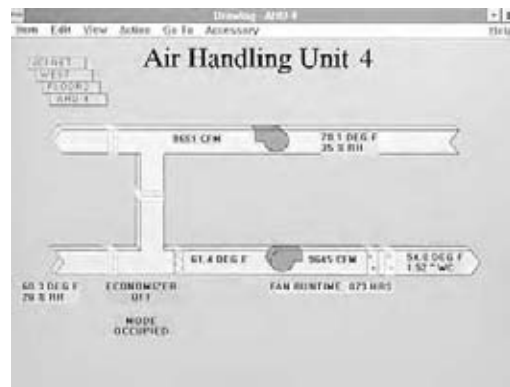
Fig. 30.33 Any workstation screen can display any portion of any system in the BAS. Here an air-handling unit (AHU) is displayed with data on airflow, air temperatures, and relative humidity in each duct section. In addition, cumulative fan run time, economizer status, and area occupancy status are displayed. (Courtesy of Johnson Controls.)
