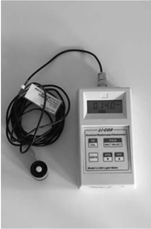
Fig. 11.9 Digital meter (from Li-Cor) has a variety of sensors that measure illuminance, solar irradiance, or photosynthetic radiation. Due to its small size, the illuminance sensor can be easily used for architectural model measurements. (Photo by Jonathan Meendering.)
