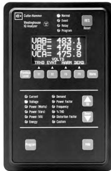
Fig. 25.24 Power system analysis unit designed to be mounted permanently into a system switchboard (see Chapter 26). This programmable unit can meter circuit parameters, measure energy and power use, analyze power quality (including harmonic analysis), and log events. (Photo courtesy of Cutler-Hammer.)
