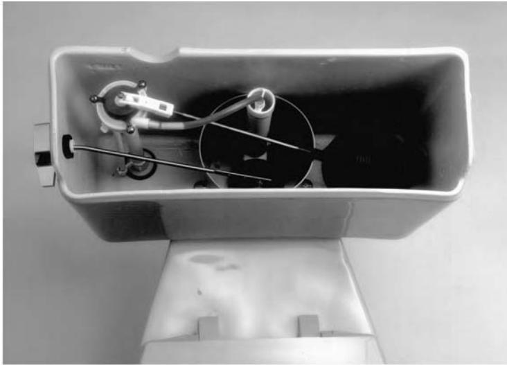
Fig. 21.47 A very-low-flow flush is achieved with a reservoir that meters about 1.4 gal (5.3 L) of water from the tank to the bowl during flushing. The standing water surface is about 4½ by 6 in. (115 by 150 mm). The Ultra-One/G. (Courtesy of Eljer Industries, Plano, TX.)
