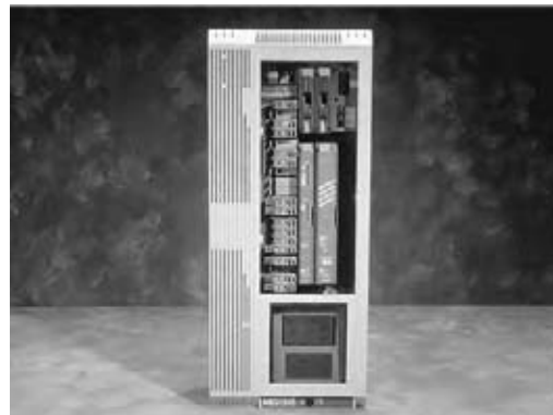
Fig. 30.37 Network control unit acts as a LAN platform, performing supervisory functions for a portion of a building. It connects to operator workstation(s) at the upper management level, to other network controllers at its level via the LAN, and to specific stand-alone controllers at the lower, control level. It can also be programmed to act as a high-quality industrial process controller. (Courtesy of Johnson Controls.)
