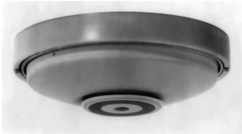
Fig. 24.51 Detectors in the illustrated design are made with fixed-temperature, nonresetting elements that melt out at 130°F (54°C) or 200°F (93°C) and rate-of-rise elements that will alarm when the temperature rise is faster than 15F° (8C°)/minute. The illustrated unit is a 200°F (93°C) fixed-temperature-only model. It is applicable to spaces with unusually violent temperature fluctuations and ceiling temperatures between 100° and 150°F (37 and 65°C). (Photo courtesy of Cerberus Pyrotechnics.)
