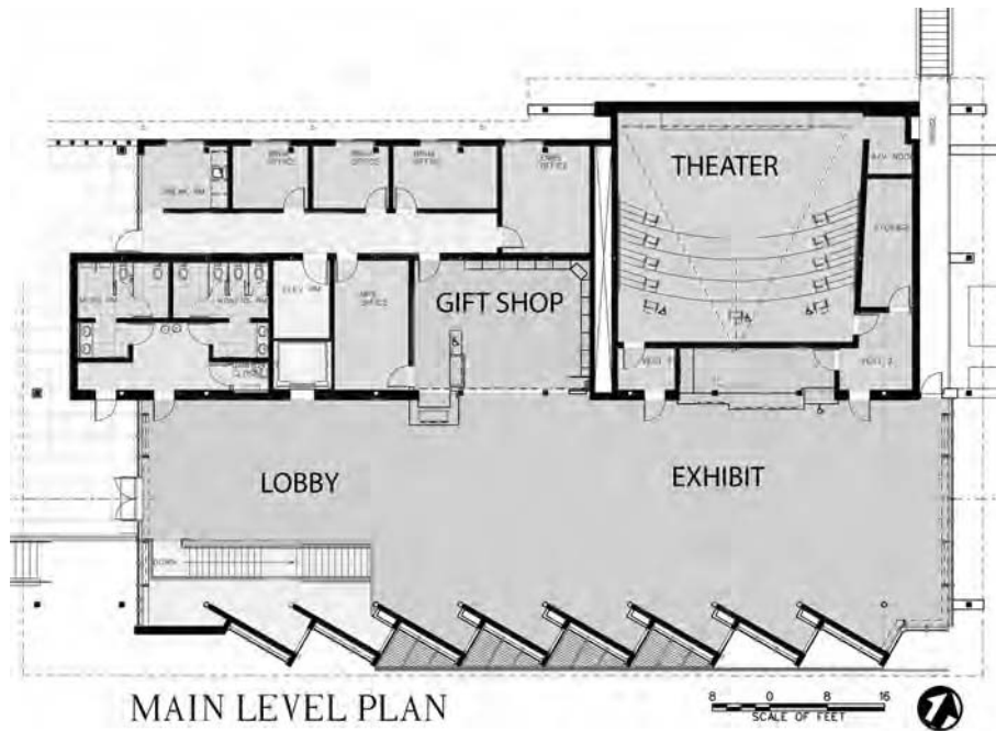
Fig. 8.60 Main floor plan showing orientation and internal organization. (© Lord, Aeck & Sargent, Inc.; used with permission.)
