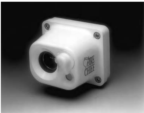
Fig. 24.50 The combined ultraviolet-infrared (UV/IR) flame detector has peak sensitivity at 200 and 4300 nm, respectively, which corresponds to the maximum emission points of a typical hydrocarbon (e.g., petroleum products) fire. This unit is equipped with a microprocessor that performs diagnostic procedures and ensures proper calibration. The detector, which measures approximately 5 × 5½ × 6 in. (127 × 144 × 152 mm) deep is suitable for use in specific class hazardous areas. (Photo courtesy of Meggitt Avionics.)
