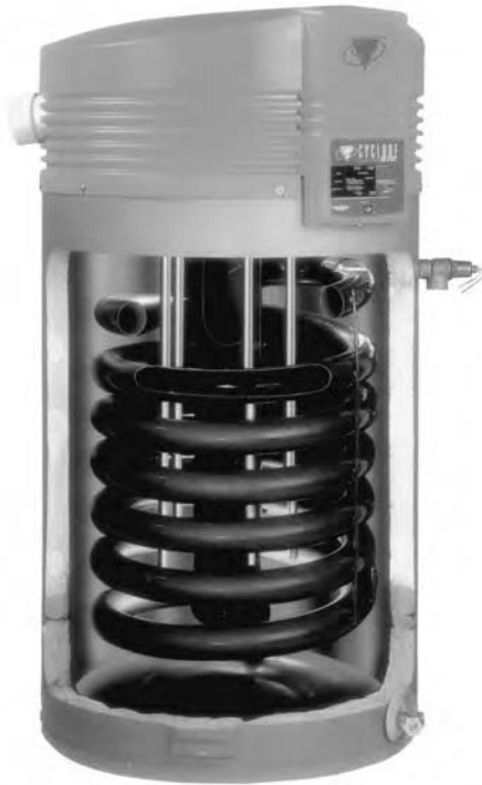
Fig. 21.22 “Cyclone XHE” water-heater storage tank using natural gas (or propane). This model achieves 94% thermal efficiency with a burner located at the top, forcing blower-driven air into a countercurrent contact with rising fuel. A precise mix of air and fuel at the point of ignition results in high combustion efficiency, and the swirling flame continues downward in a submerged central combustion chamber. The heated gas is then forced at high velocity through the spiral heat-exchanger coil, with a swirling action that maximizes heat exchange with the water. (Courtesy of the A.O. Smith Water Products Company, Irving, TX.)
