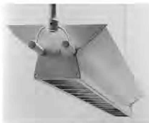
Fig. 16.17 (a) Semi-indirect, low-brightness, deep-cell parabolic baffle fluorescent fixture. The parabolic baffle provides the required low luminance in the parallel direction (see text), as does the fixture body in the normal plane, so the fixtures should not cause glare. (See luminance figures in the photometric table.) (b) Photometry. Maximum ceiling luminance and ceiling luminance ratios depend on hanger length, ceiling reflectance, and fixture spacing. (c) Photograph of a semi-indirect luminaire showing construction and suspension hardware. (Courtesy of Zumtobel-STAFF Lighting Co.)
