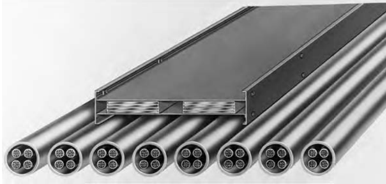
Fig. 27.9 Sectional view of a busduct (on top) shows the tight assembly of insulated conductors within a metal housing. This design, unlike the ventilated type, can be mounted in any position because heat dissipation is by conduction from the busbars to the housing. The eight sets of cable shown beneath it have the same current-carrying capacity as the busduct. (Reproduced by permission of Square D Company.)
