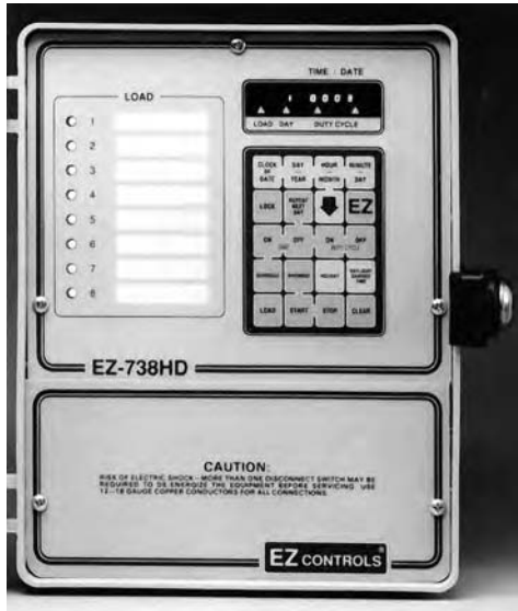
Fig. 26.14 Programmable time switch. This unit, which measures 9.5 in. H x 8 in. W x 4.5 in. D (240 x 200 x 115 mm) in its cabinet, permits independent programming of eight 20-A, 240-V circuits. Each circuit (channel) can be arranged for multiple on-off daily operations and can be programmed on a 7-day-a-week basis, with special 365-day functions such as automatic daylight saving time adjustment. (Courtesy of EZ Controls.)
