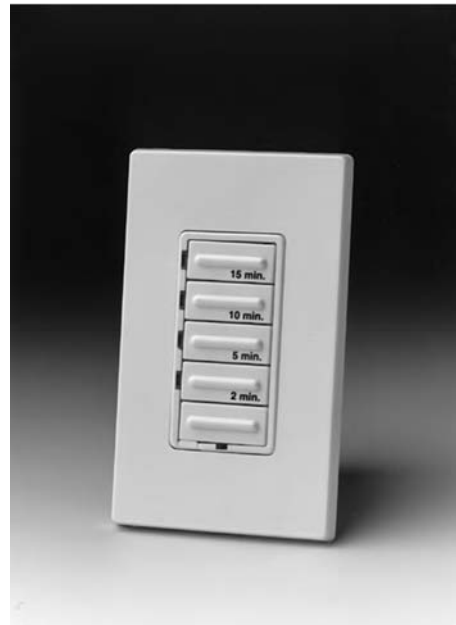
Fig. 26.48 Solid-state adjustable electronic switch timer that mounts in a common wall-switch box. The unit switches off, with delay adjustable from zero to 15 minutes in five discrete steps. Units such as these can control incandescent and fluorescent lamps and small motors. They are applicable where either direct manual control or occupancy sensors are inapplicable. (Photo courtesy of Leviton Manufacturing Co.)
