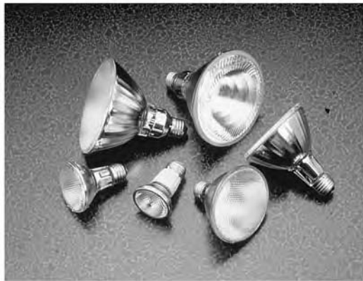
Fig. 12.12 PAR halogen lamp with standard medium screw bases in sizes PAR 16, 20, 30, and 38 with a short or elongated lamp neck. Lamp wattages range from 45 to 90 W. (Courtesy of Philips Lighting Co.)
