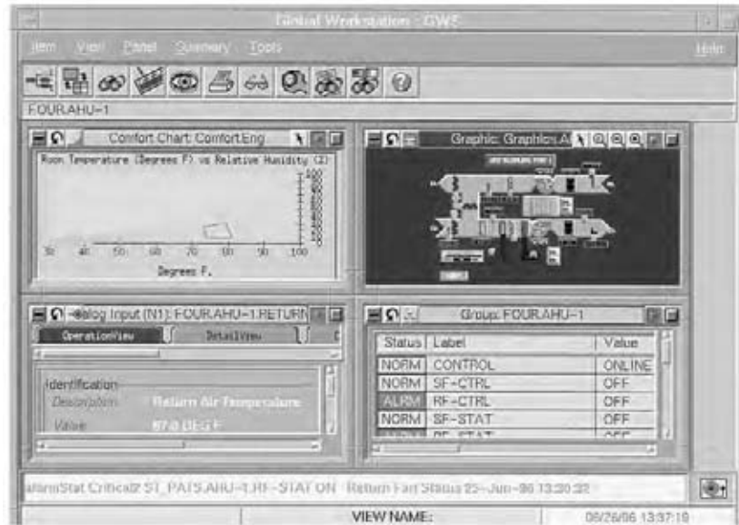
Fig. 30.34 Global workstation screen is arranged to display four separate data windows. Clockwise from upper left: (1) Comfort chart showing a plot of room psychrometric conditions on a graph of room temperature versus relative humidity. (2) Graphic screen showing the layout of an AHU with relevant data. (3) Status chart of items in AHU-1. (4) Temperature readout of return air for AHU-1. (Courtesy of Johnson Controls.)
