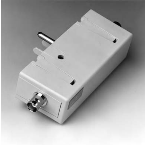
Fig. 26.65 TVSS device designed to protect video lines from voltage transients. The unit plugs into a standard outlet to establish a ground connection for current bypass. This unit is equipped with BNC (Bayonet Neill-Concelman) connections; others have telephone, PL (coaxial), and RS (serial device) connectors for use on telephone, communication, and data lines. The illustrated unit has a clamping voltage of 15 V and a maximum surge current capacity of 5000 A. It measures approximately 2 in. W × 4 in. H × 1 in. D (50 × 100 × 25 mm). (Photo courtesy of Leviton Manufacturing Co.)
