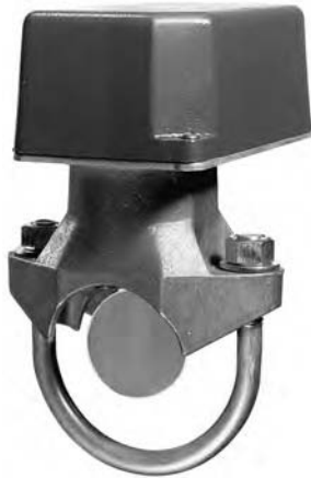
Fig. 24.59 Typical water flow indicator. The unit bolts onto a sprinkler pipe with the paddle inside the pipe. Any water motion deflects the paddle, causing a signal to be transmitted from the microswitch mounted in the box on top of the pipe. (Courtesy of Simplex/Potter.)
