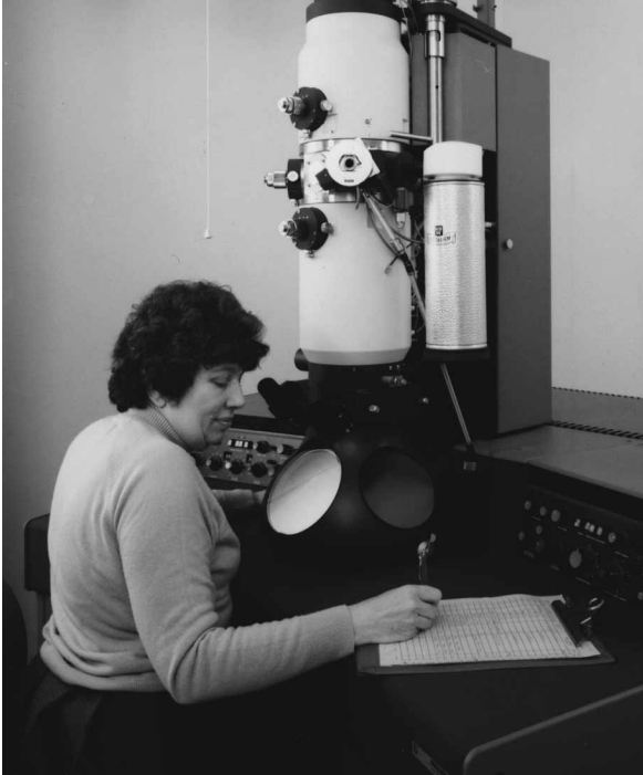
Figure 4.4. Dr. Anne Field at a Philips 420 transmission electron microscope. Courtesy of Mr. J. Gibson.
