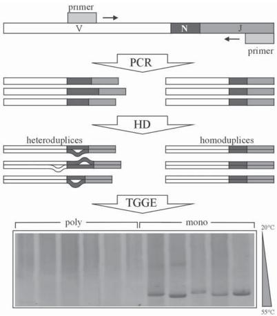
Fig. 2. Principles of TCRγ-PCR with subsequent HD-TGGE.
