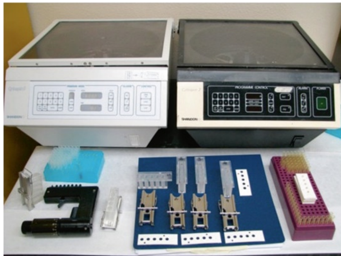
Equipment needed: Cytospins, "multi-spot" cuvettes and filter papers
