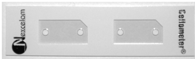
Fig. 3. Cellometer counting chamber – each slide has two counting chambers which can be filled in the hood, and in our hands this has proved much quicker and cleaner than haemocytometer counting methods. For details see http://www.nexcelom.com .
