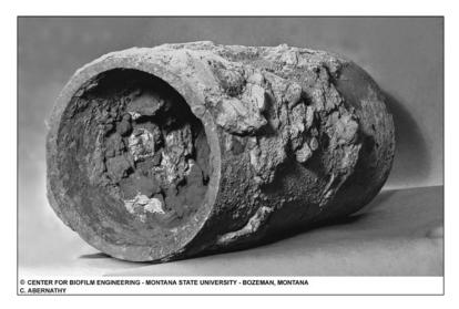
Figure 4.2 Biofilm corrosion. This pipe has been almost completely occluded by biofilm, which has dried and hardened. Few technologies exist for removing biofilm from living or nonliving surfaces. (Courtesy of Center for Biofilm Engineering, Montana State University)
