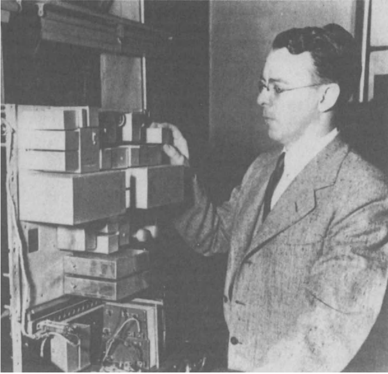
Figure 10.2. H. S. Black and a 1930 negative feedback repeater.
