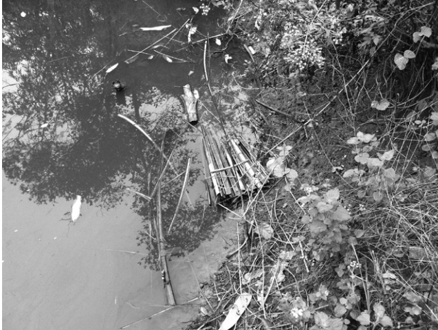
16.3 Wood and bamboo soaking in a pond at edge of a rice paddy field.
