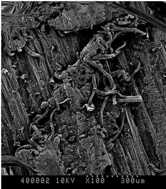
23.7 Welded bondline. Note the entangled wood cells (fibers) immersed in a mass of molten material. The whole superimposed on a background of elongated, undamaged, wood cells.
