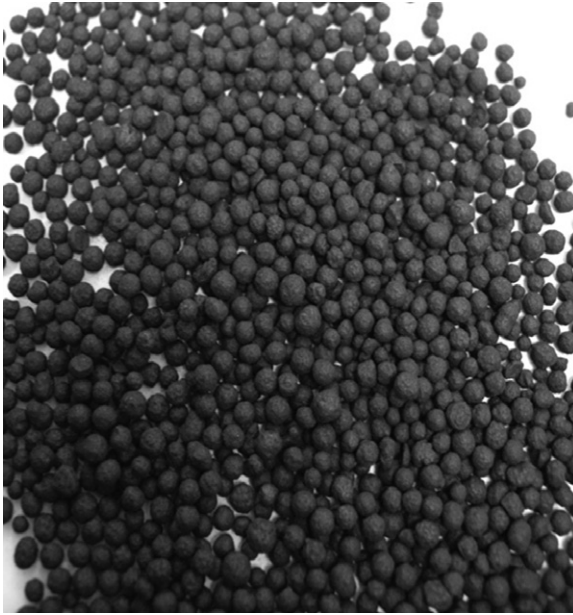
16.16 Slow release fertiliser produced from Biochar, minerals and a source of N.
