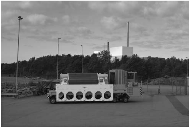
14.8 Transport container TN17 for spent nuclear fuel (© SKB).
