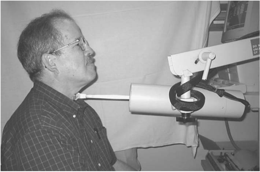
Figure 1. Illustration of the basic setup used to measure thyroid uptake (Radioactive Iodine Uptake, RAIU).
